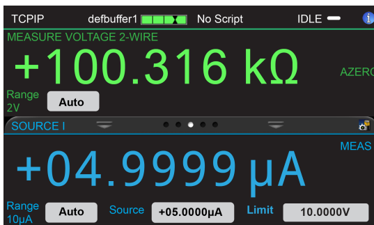
Figure 66: Resistance measurement SIMV and read ohms
