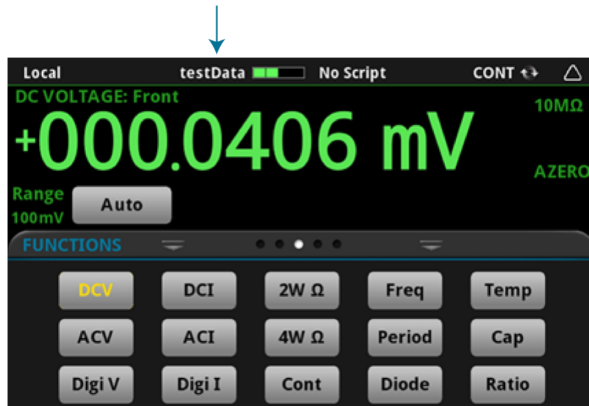
Figure 131: Active buffer indicator
