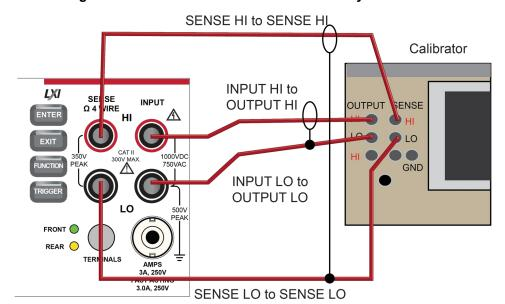
Figure 7: Connections for 4-wire RTD accuracy verification
