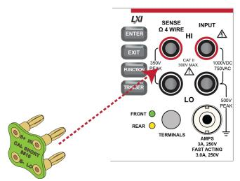
Figure 17: Front panel 4-wire shorting plug orientation
