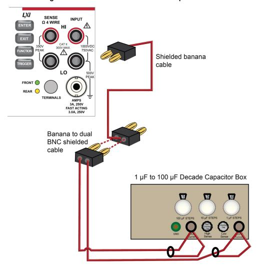
Figure 15: Connect DMM6500 to decade capacitor box
