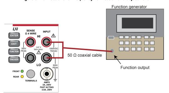
Figure 5: Connections for frequency verification and adjustment
