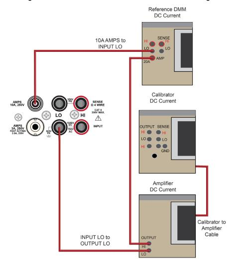
Figure 18: Connections for dc current verification 10 A range
