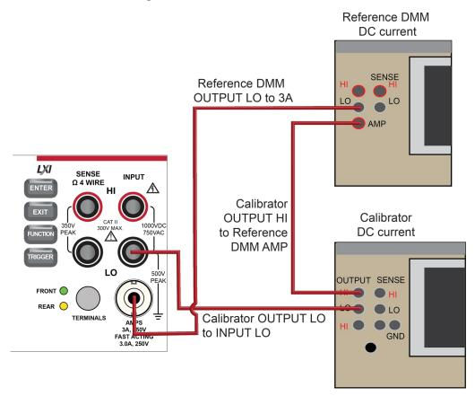
Figure 11: Connection for dc current
