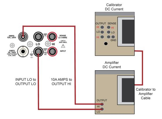
Figure 19: Connections for the 10 A range
