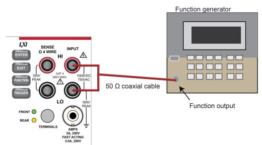
Figure 30: Connection for a frequency adjustment
