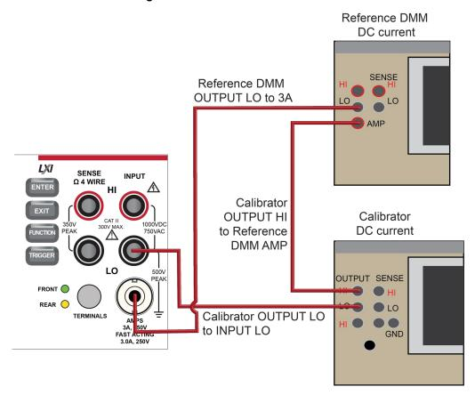
Figure 25: Connection for dc current
