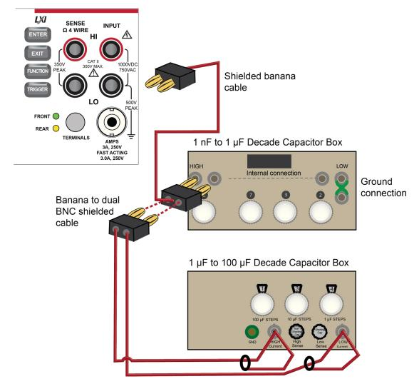
Figure 16: Capacitance verification connections
