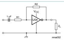
Maximum  $V_{o(p-p)} = V_{CC} - 1.5 \text{ V}$  centered at  $0.5 \times V_{CC}$ .
