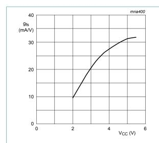
Typical forward transconductance gfs as a function of the supply voltage at T<sub>amb</sub> = 25 °C
