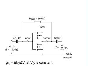
Test set-up for measuring forward Fig. 7. transconductance
