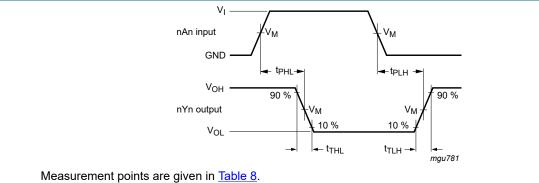
$V_{\text{OL}}$  and  $V_{\text{OH}}$  are typical voltage output drop that occur with the output load.
