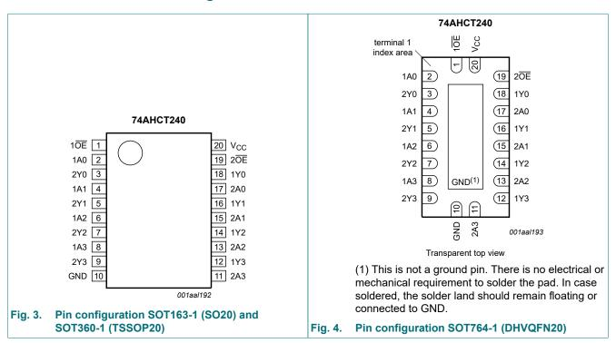
Octal buffer/line driver; inverting; 3-state
