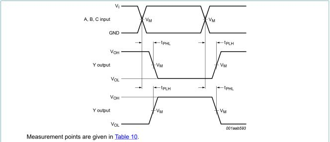
$V_{\text{OL}}$  and  $V_{\text{OH}}$  are typical output voltage levels that occur with the output load.
