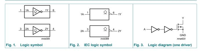
Low-power dual inverter with open-drain output
