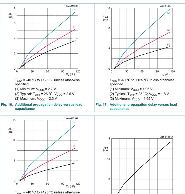
$T_{amb} = -40^{\circ}$  C to +125 °C unless otherwise specified. (1) Minimum: V<sub>CCO</sub> = 1.6 V
