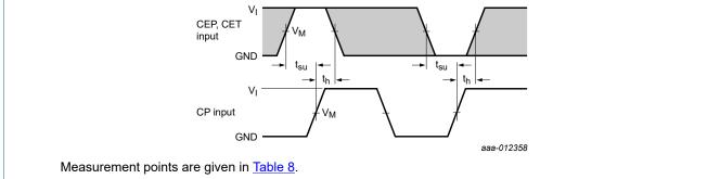
The shaded areas indicate when the input is permitted to change for predictable output performance.
