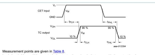
Logic levels V<sub>OL</sub> and V<sub>OH</sub> are typical output voltage levels that occur with the output load.
