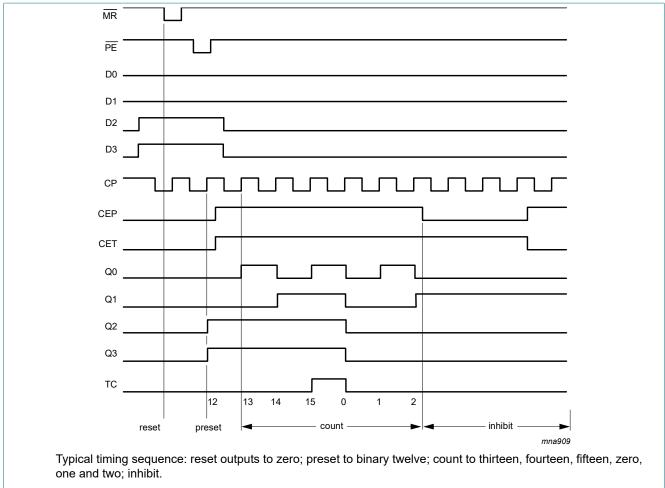
Fig. 8. Typical timing sequence
