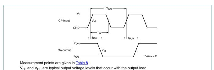
Fig. 6. Propagation delay clock (CP) to output (Qn), clock pulse width and maximum clock frequency
