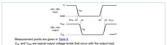
Fig. 4. The input (nAn, nBn) to output (nBn, nAn) propagation delays
