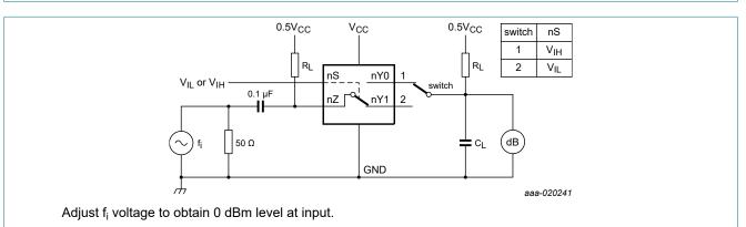
Fig. 19. Test circuit for measuring isolation (OFF-state)
