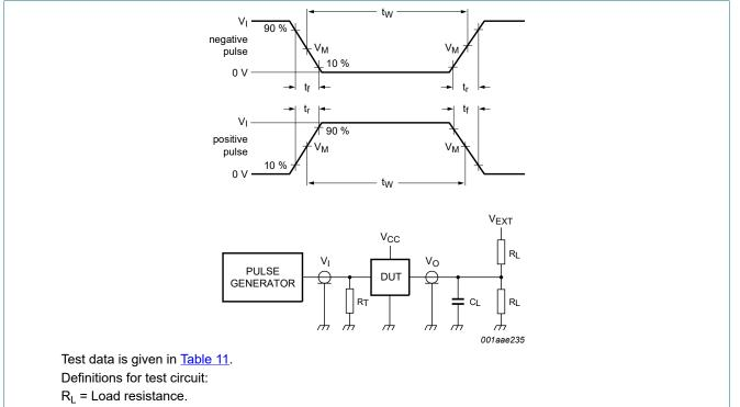
C<sub>L</sub> = Load capacitance including jig and probe capacitance.
