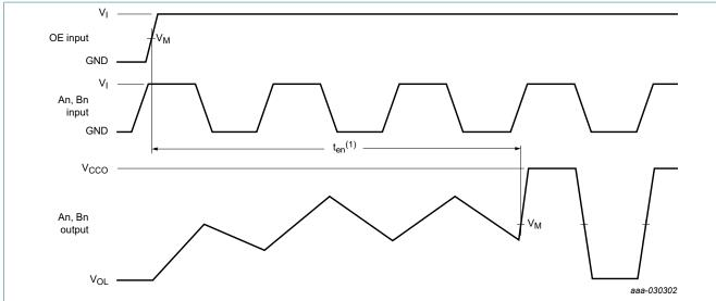
(1) The enable time  $(t_{en})$  indicates the amount of time the user must allow for one one-shot circuitry to become operational after OE is taken HIGH. See also Section 12.6
