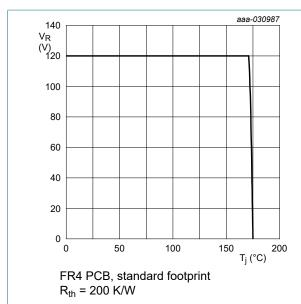
Fig. 11. Derated maximum reverse voltage as a function | Fig. 12. Derated maximum reverse voltage as a function of junction temperature; typical values
