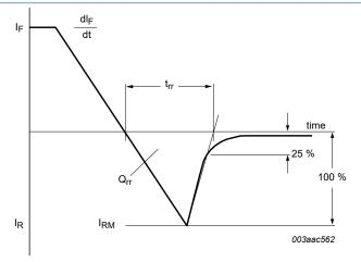
Fig. 15. Reverse recovery definition; ramp recovery
