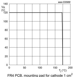
FR4 PCB, mounting pad for cathode 1 cm<sup>2</sup>  $R_{th} = 120 \text{ K/W}$
