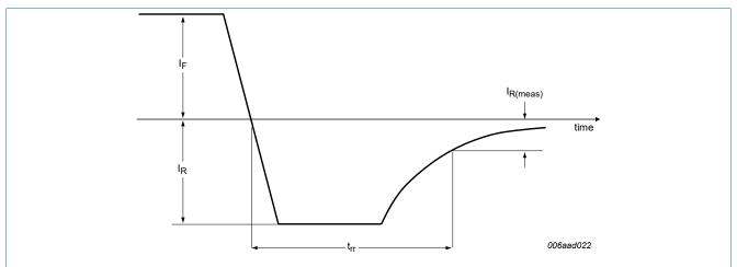
Fig. 14. Reverse recovery definition; step recovery
