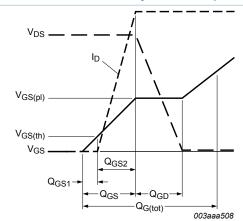
Fig. 13. Gate charge waveform definitions
