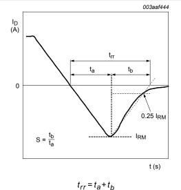
Fig. 16. Reverse recovery waveform definitions
