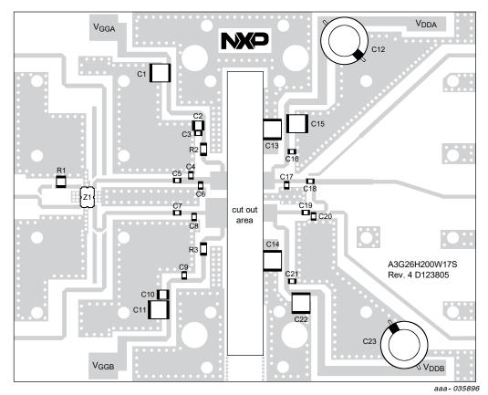
Figure 2. A3G26H200W17S Production Test Circuit Component Layout
