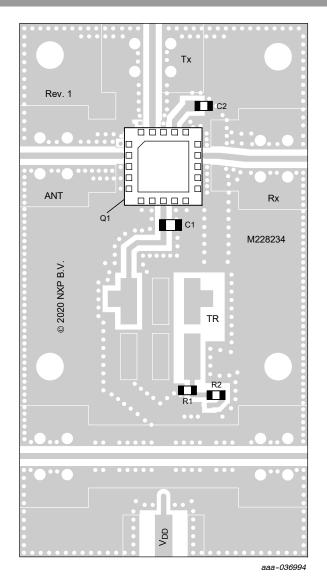
Figure 3. AFRX5G372 Application Circuit Component Layout
