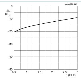
Diode zero-biased and inserted in series with a 50  $\Omega$  strip line circuit and biased via the analyzer T-network; T<sub>amb</sub> = 25 °C
