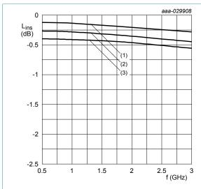
Diode inserted in series with a 50  $\Omega$  strip line circuit and biased via the analyzer T-network;  $T_{amb}$  = 25 °C;
