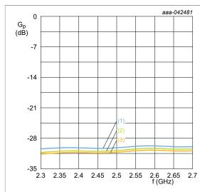
Figure 23. TX bypass mode, Gp versus frequency over temperature
