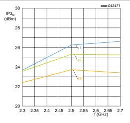
Figure 17. Low gain RX mode, IP3<sub>o</sub> versus frequency over temperature
