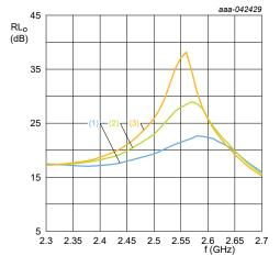
Figure 7. High gain RX mode, RL<sub>o</sub> versus frequency over temperature
