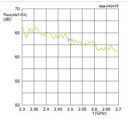
Figure 22. TX mode, ANT to RX\_OUT isolation versus frequency
