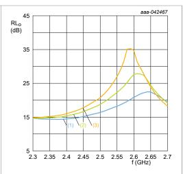
Figure 15. Low gain RX mode, RL<sub>o</sub> versus frequency over temperature
