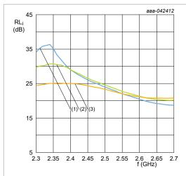
Figure 6. High gain RX mode, RL<sub>i</sub> versus frequency over temperature
