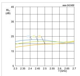
Figure 14. Low gain RX mode, RL<sub>i</sub> versus frequency over temperature
