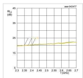
Figure 21. TX mode,  $RL_o$  versus frequency over temperature
