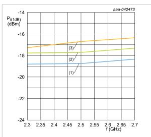
Figure 18. Low gain RX mode, Input P<sub>i(1dB)</sub> versus frequency over temperature
