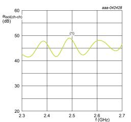
Figure 11. High gain RX mode, Channel Isolation versus frequency
