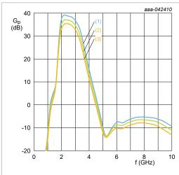
Figure 4. High gain RX mode,  $\mathbf{G}_{\mathbf{p}}$  versus frequency over temperature
