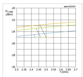
Figure 10. High gain RX mode,  $P_{i(1dB)}$  versus frequency over temperature
