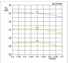
Figure 13. Low gain RX mode,  $\mathbf{G}_{\mathrm{p}}$  versus frequency over temperature
