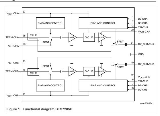
2.3 GHz - 2.7 GHz RX Analog Front-End Module with bypass
