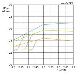
Figure 9. High gain RX mode, IP3<sub>o</sub> versus frequency over temperature
