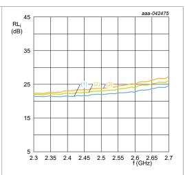
Figure 20. TX mode,  $RL_i$  versus frequency over temperature
