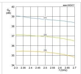
Figure 5. High gain RX mode,  $\mathbf{G}_{\mathbf{p}}$  versus frequency over temperature
