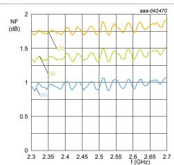
Figure 16. Low gain RX mode, NF versus frequency over temperature
