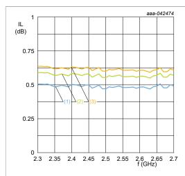
Figure 19. TX mode,  $\alpha_{\text{ins}}$  versus frequency over temperature
