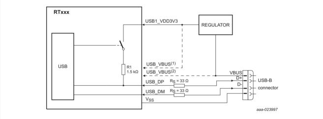
Two options exist for connecting VBUS to the USB\_VBUS pin:
