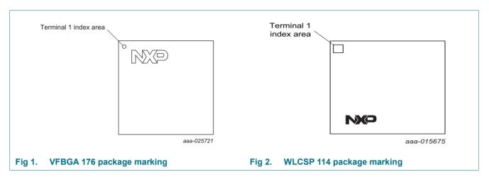
The MIMXRT6xxSFAWBR WLCSP114 production samples has the following top-side package marking:
