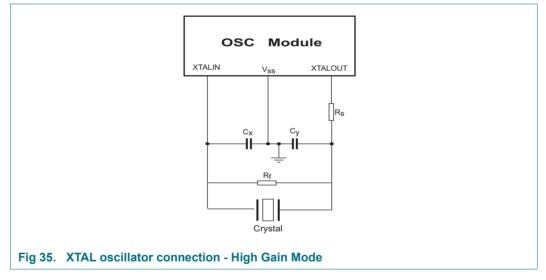
For best results, it is very critical to select a matching crystal for the on-chip oscillator. Load capacitance (CL), series resistance (RS), and drive level (DL) are important parameters to consider while choosing the crystal. After selecting the proper crystal, the approximate external load capacitor  $C_x$  and  $C_y$  values can also be generally determined by the following expression:
