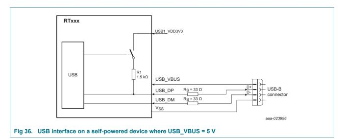
The internal pull-up  $(1.5 \text{ k}\Omega)$  can be enabled by setting the DCON bit in the DEVCMDSTAT register to prevent the USB from timing out when there is a significant delay between power-up and handling USB traffic. External circuitry is not required.
