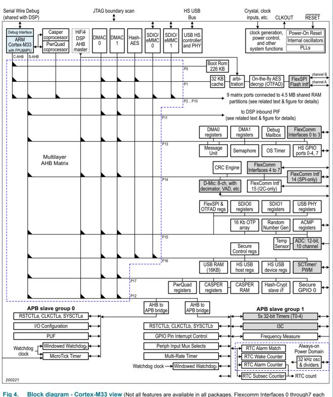
include USART, SPI, I2C, and I2S functions. Grey-shaded blocks indicate peripherals that provide DMA requests or are otherwise able to trigger DMA transfers. Hash-AES and SDIO include a dedicated DMA function.)
