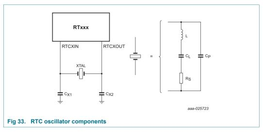
For best results, it is very critical to select a matching crystal for the on-chip oscillator. Load capacitance (CL), series resistance (RS), and drive level (DL) are important parameters to consider while choosing the crystal. After selecting the proper crystal, the approximate external load capacitor Cx and Cy values can also be generally determined by the following expression:
