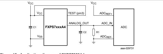
Figure 12. Application diagram of FXPS7250A4
