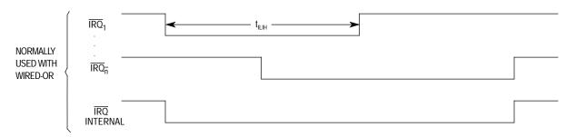
b. Level-Sensitive Trigger Condition. If after servicing an interrupt the  $\overline{\mbox{IRQ}}$  remains low, the next interrupt is recognized.
