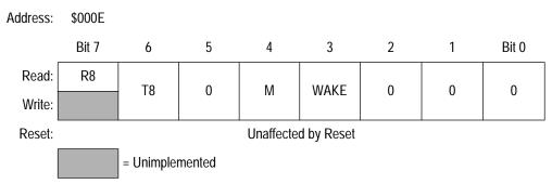
Figure 9-5. SCI Control Register (SCCR1)
