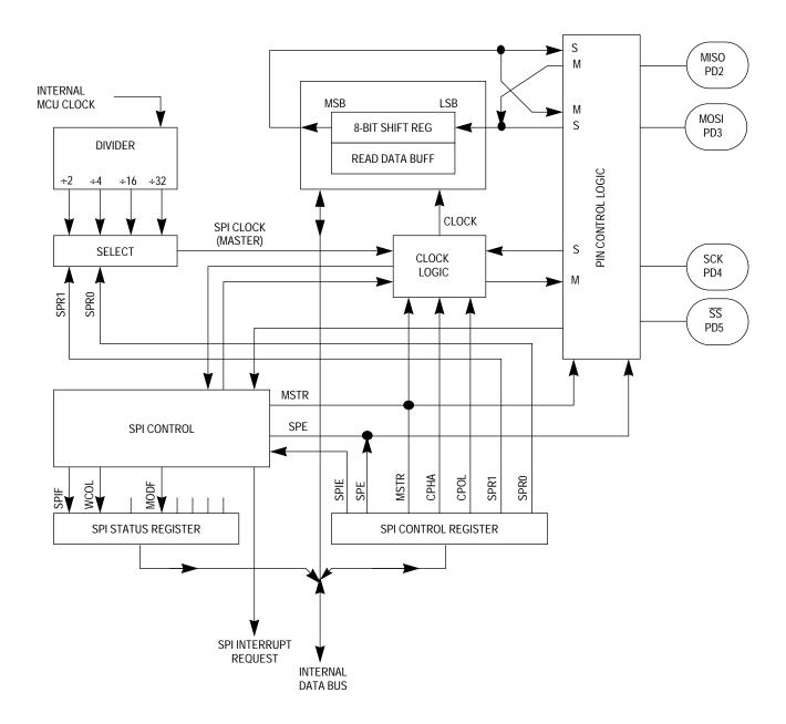
Figure 10-2. Serial Peripheral Interface Block Diagram
