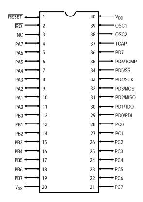
Figure 11-1. User Mode Pinout
