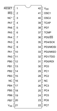
$<sup>^{\</sup>star}\,$  If MC68HC705C4A OTPs are to be used in the same application, this pin should be tied to  $V_{DD}.$
