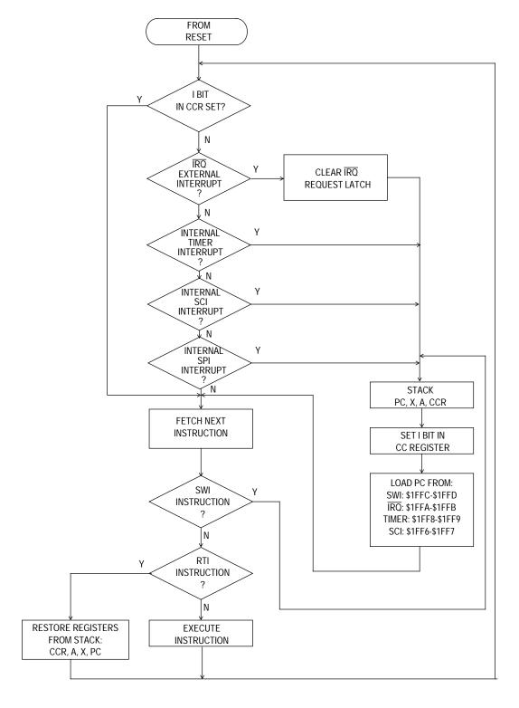
Figure 4-1. Interrupt Flowchart
