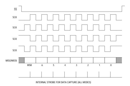
Figure 10-1. Data Clock Timing Diagram
