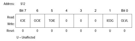
Figure 8-4. Timer Control Register (TCR)
