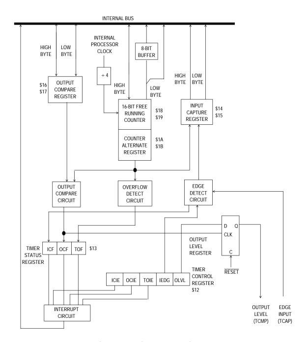
Figure 8-1. Timer Block Diagram
