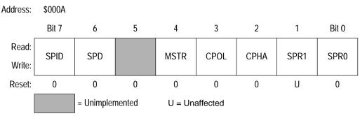
Figure 10-4. SPI Control Register (SPCR)
