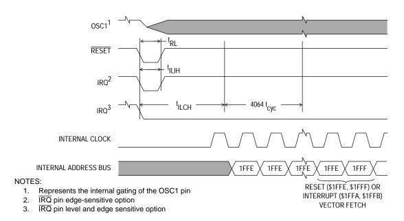
Figure 6-2. Stop Recovery Timing Diagram
