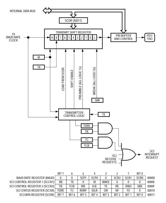
Figure 9-2. SCI Transmitter
