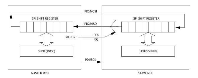
Figure 10-3. Serial Peripheral Interface Master-Slave Interconnection
