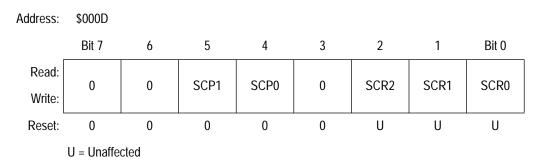
Figure 9-8. Baud Rate Register (BAUD)
