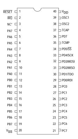
$<sup>^{\</sup>star}\,$  If MC68HC705C4A OTPs are to be used in the same application, this pin should be tied to  $V_{DD}.$
