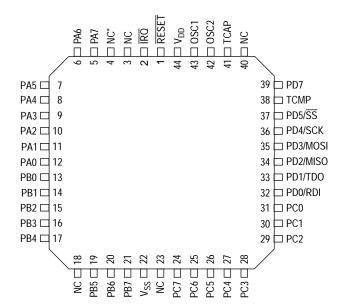
$<sup>^{\</sup>star}\,$  If MC68HC705C4A OTPs are to be used in the same application, this pin should be tied to  $V_{DD}.$
