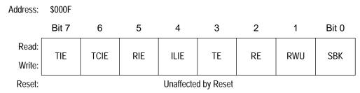
Figure 9-6. SCI Control Register 2 (SCCR2)
