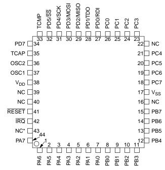
$<sup>^{\</sup>star}$  If MC68HC705C4A OTPs are to be used in the same application, this pin should be tied to  $V_{DD}.$
