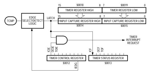
Figure 8-3. Input Capture Operation
