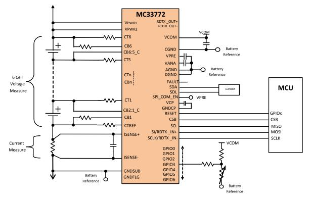
Figure 1. Simplified application diagram of SPI communication context
