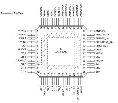
Figure 4. 33772 pinout diagram
