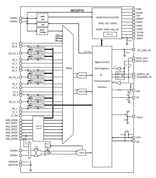
Figure 3. Simplified internal block diagram
