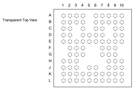
Figure 3. MR2001T pinout (ball) diagram
