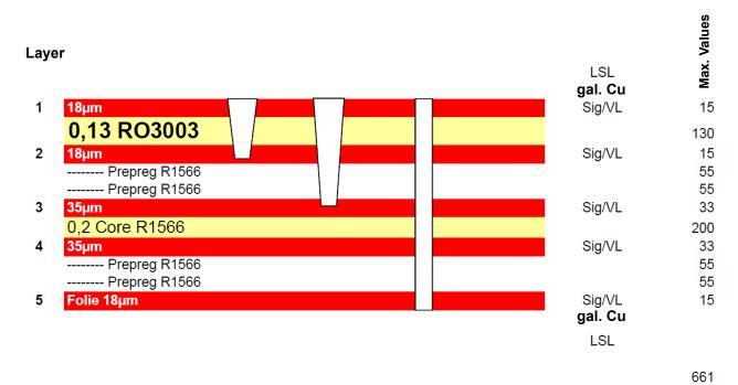
Figure 23. RO3003 on top of a FR4 core
