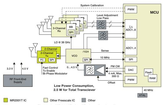
Figure 1. MR2001T simplified application diagram
