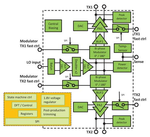
Figure 2. MR2001T two-channel transmitter block diagram
