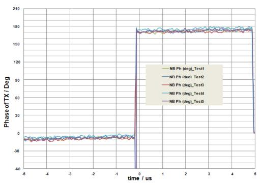
Figure 18. Bi-phase modulator switching time
