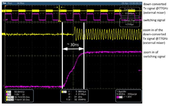
Figure 17. Switching of the Tx output signal at 77 GHz using the dedicated fast control signals
