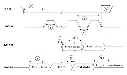
Figure 7. Typical SPI timing chart
