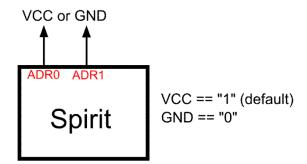
Figure 8. External connection of address pins ADR0 and ADR1 to define the identification key of the chip
