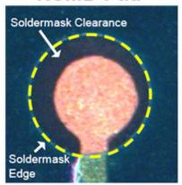
Figure 28. Solder mask (SMD) and non-solder mask defined (NSMD) pads
