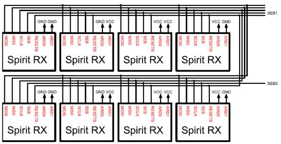
Figure 10. Typical Rx chip partitioning for more than four receivers. individual SEB signals for more than four Rx chips are required
