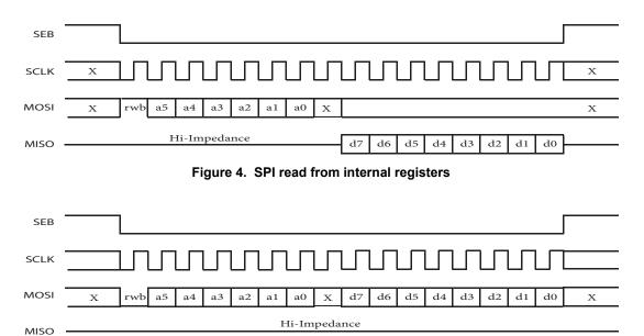
Figure 5. SPI write to internal registers
