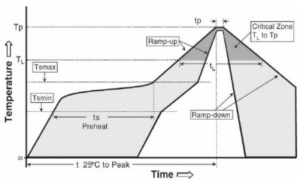
Figure 29. Typical MR2001 reflow profile
