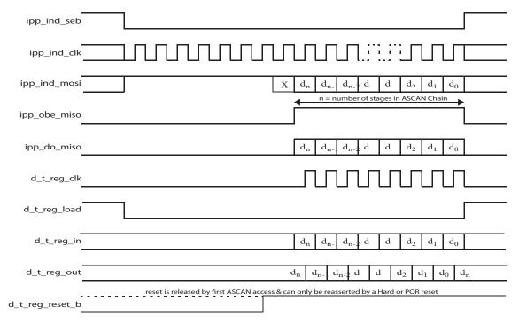
Figure 6. SPI write/read to ASCAN
