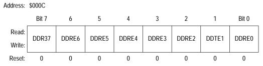
Figure 15. Data Direction Register E (DDRE)
