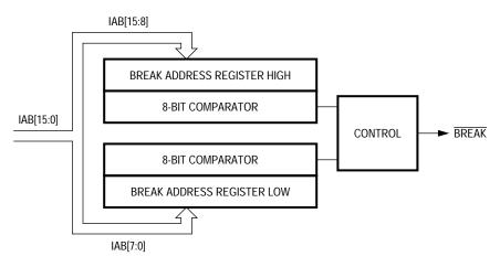
Figure 1. Break Module Block Diagram
