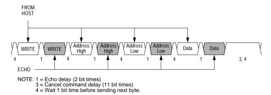
Figure 5. Write Transaction
