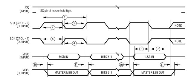
NOTE: This last clock edge is generated internally, but is not seen at the SCK pin.
