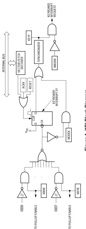
Figure 1. KBI Block Diagram
