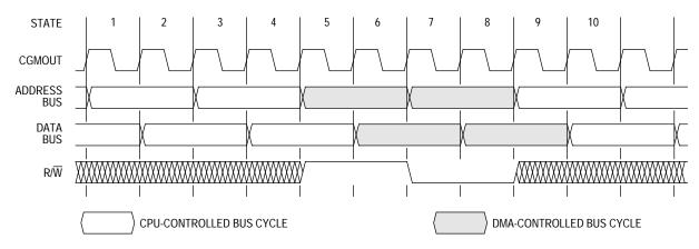
Figure 3. Single Byte Transfer Timing (Any DMA Bus Bandwidth)
