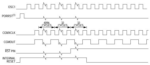
1. PORRST is an internally generated power-on reset pulse.
