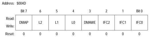
Figure 18. DMA Status and Control Register (DSC)
