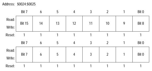
Figure 7. TIM Counter Modulo Registers (TMODH and TMODL)
