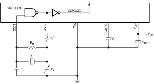
\*R<sub>S</sub> can be 0 (shorted) when used with higher-frequency crystals. Refer to manufacturer's data.
