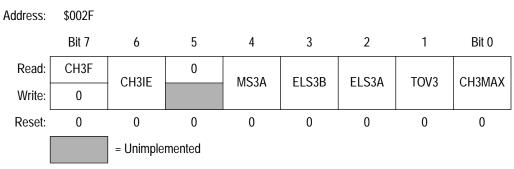
Figure 11. TIM Channel 3 Status and Control Register (TSC3)
