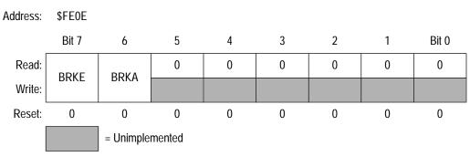
Figure 3. Break Status and Control Register (BSCR)
