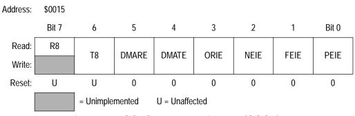
Figure 13. SCI Control Register 3 (SCC3)
