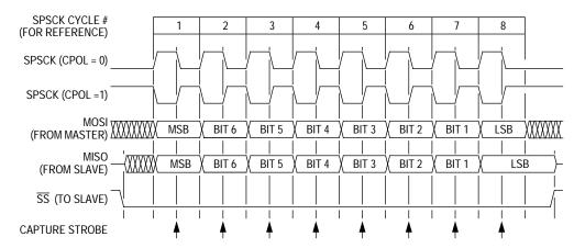
Figure 6. Transmission Format (CPHA = 1)
