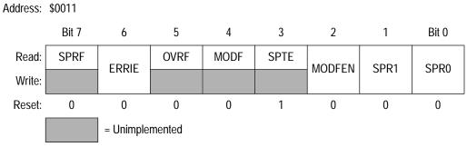
Figure 15. SPI Status and Control Register (SPSCR)
