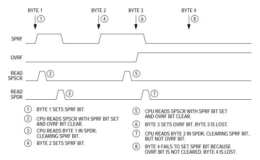
Figure 10. Missed Read of Overflow Condition
