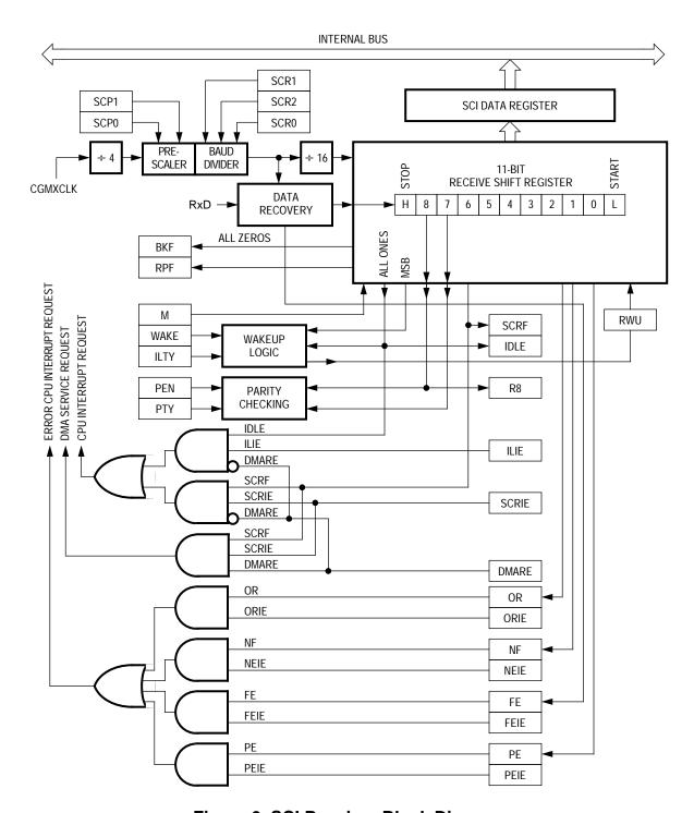
Figure 6. SCI Receiver Block Diagram
