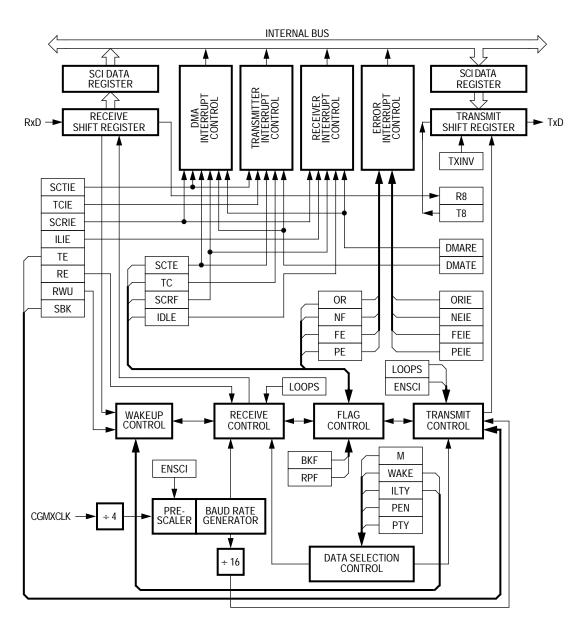
Figure 1. SCI Module Block Diagram
