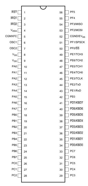
Figure 2. SDIP Pin Assignments
