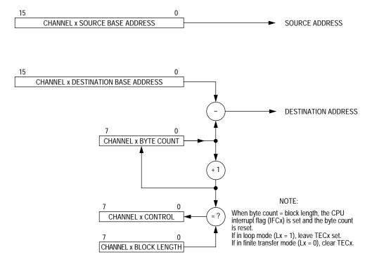
Figure 7. Static Source and Decremented Destination
