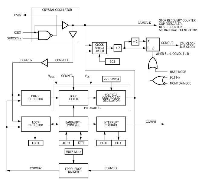
Figure 1. CGM Block Diagram
