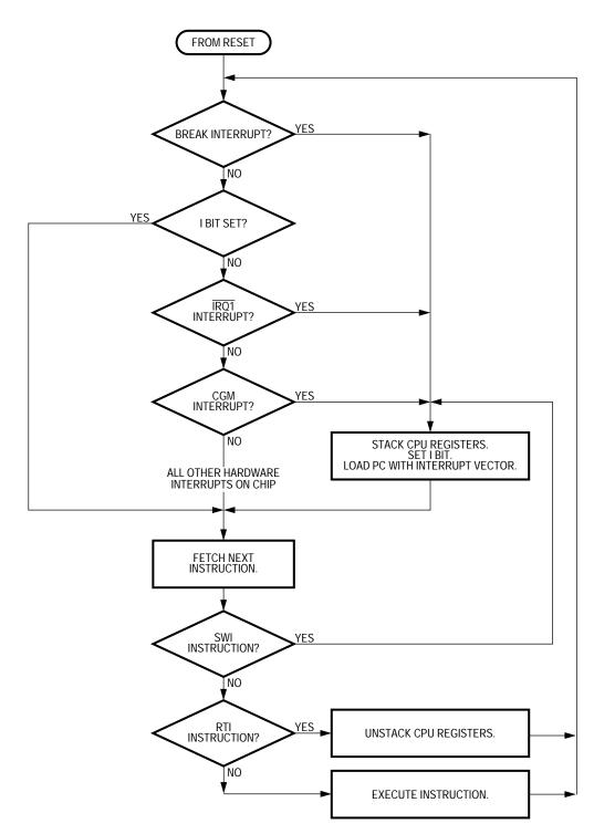
**Figure 6. Interrupt Processing**
