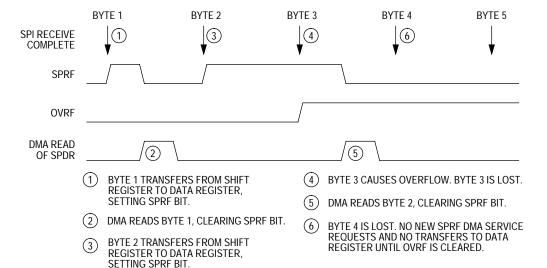
Figure 9. Overflow Condition with DMA Service of SPRF
