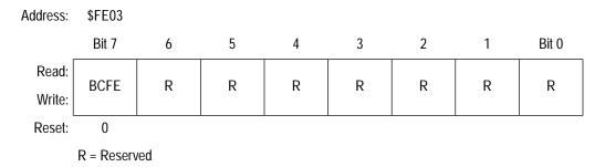
Figure 6. Break Flag Control Register (BFCR)
