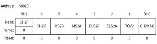
Figure 10. TIM Channel 2 Status and Control Register (TSC2)
