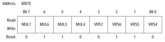
Figure 6. PLL Programming Register (PPG)
