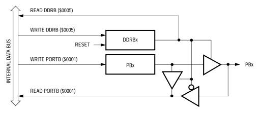
Figure 7. Port B I/O Circuit
