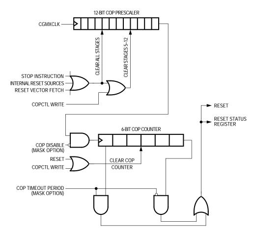
Figure 1. COP Block Diagram
