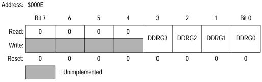
Figure 21. Data Direction Register G (DDRG)
