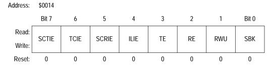
Figure 12. SCI Control Register 2 (SCC2)
