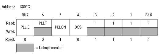
Figure 4. PLL Control Register (PCTL)
