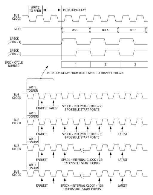
Figure 7. Transmission Start Delay (Master)
