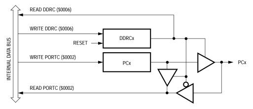
Figure 10. Port C I/O Circuit
