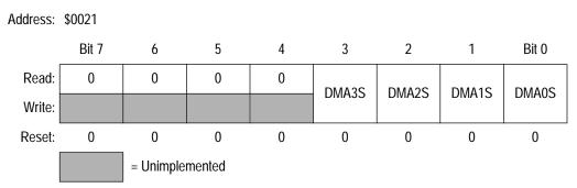
Figure 5. TIM DMA Select Register (TDMA)
