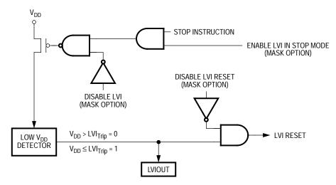
Figure 1. LVI Module Block Diagram
