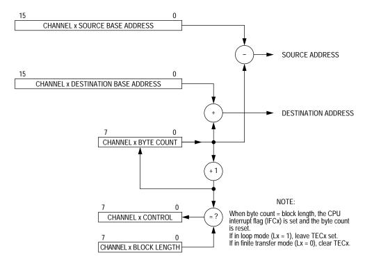
Figure 11. Decremented Source and Incremented Destination
