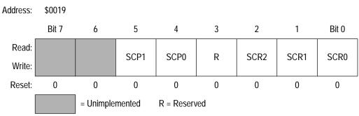
Figure 18. SCI Baud Rate Register (SCBR)
