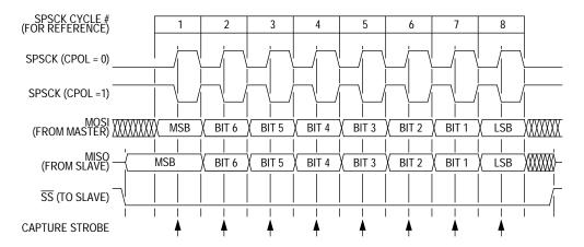
Figure 4. Transmission Format (CPHA = 0)
