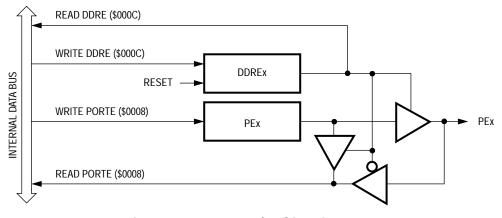
Figure 16. Port E I/O Circuit
