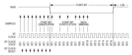
Figure 8. Receiver Data Sampling
