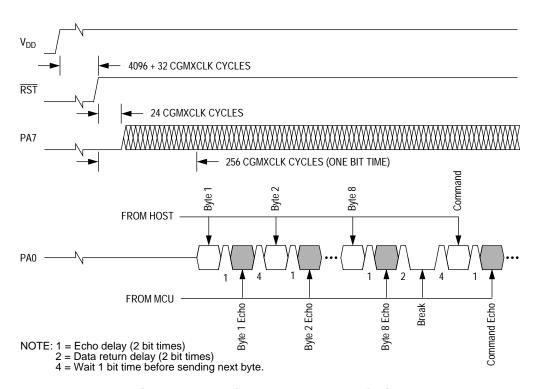
Figure 7. Monitor Mode Entry Timing
