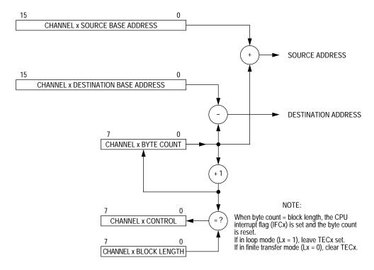
Figure 12. Incremented Source and Decremented Destination
