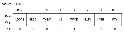
Figure 11. SCI Control Register 1 (SCC1)
