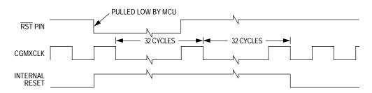
Figure 1. Internal Reset Timing
