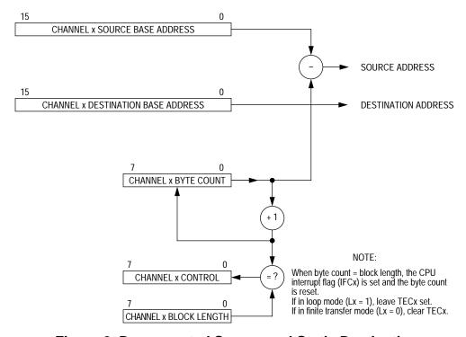
Figure 8. Decremented Source and Static Destination
