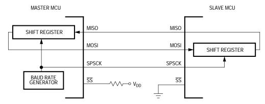
Figure 3. Full-Duplex Master-Slave Connections
