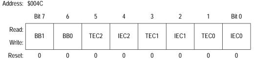
Figure 14. DMA Control Register 1 (DC1)
