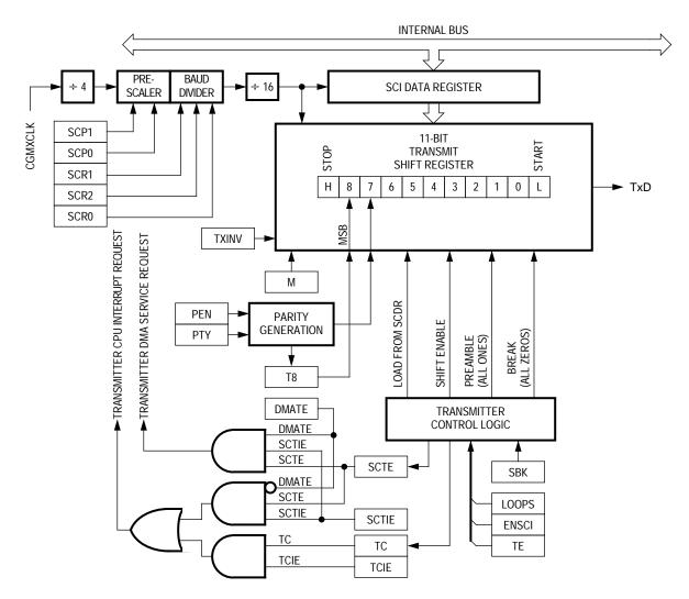
Figure 4. SCI Transmitter
