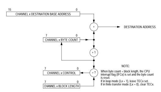
Figure 9. Static Source and Incremented Destination
