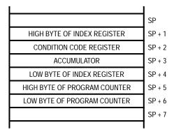
Figure 6. Stack Pointer at Monitor Mode Entry
