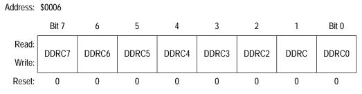
Figure 9. Data Direction Register C (DDRC)
