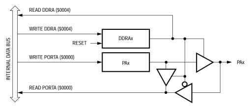
Figure 4. Port A I/O Circuit
