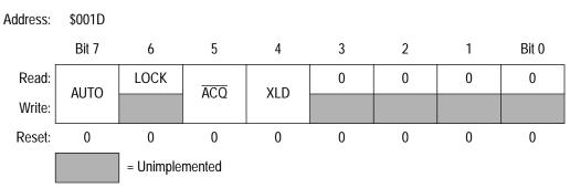
Figure 5. PLL Bandwidth Control Register (PBWC)
