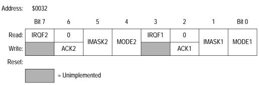
Figure 2. IRQ Status and Control Register (ISCR)
