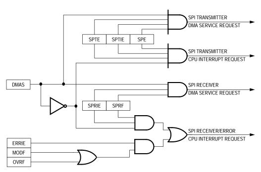
Figure 12. SPI Interrupt Request Generation
