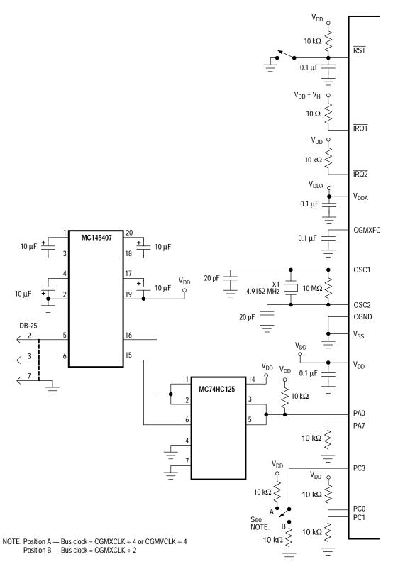
**Figure 1. Monitor Mode Circuit**
