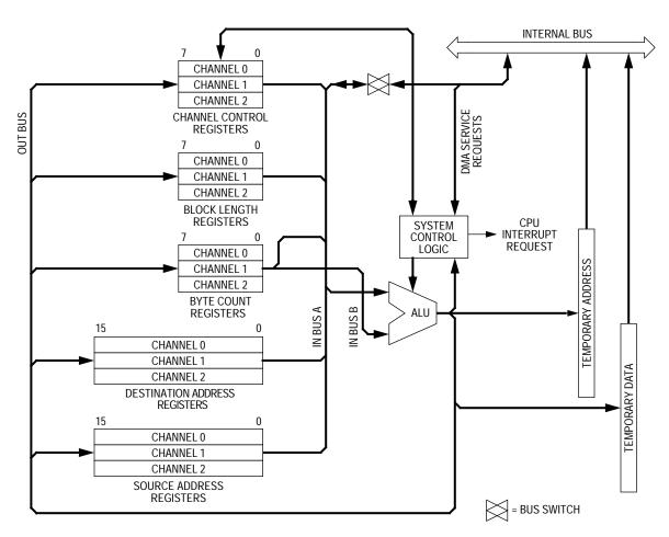
Figure 1. DMA Module Block Diagram
