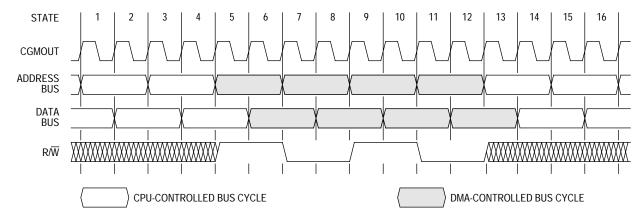
Figure 4. Single Word Transfer Timing (100% DMA Bus Bandwidth)
