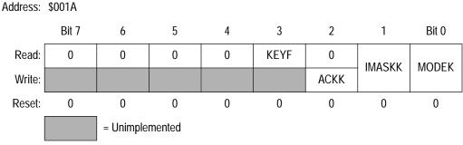
Figure 3. Keyboard Status and Control Register (KBSCR)
