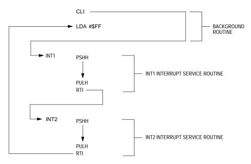
Figure 5. Interrupt Recognition Example
