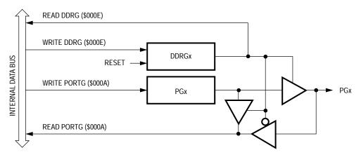
Figure 22. Port G I/O Circuit
