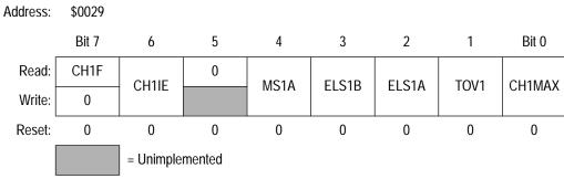
Figure 9. TIM Channel 1 Status and Control Register (TSC1)
