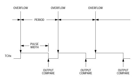
Figure 3. PWM Period and Pulse Width
