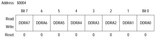
Figure 3. Data Direction Register A (DDRA)
