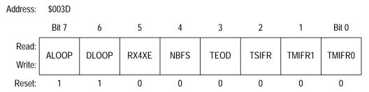
Figure 20-18. BDLC Control Register 2 (BCR2)
