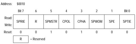
Figure 18-13. SPI Control Register (SPCR)
