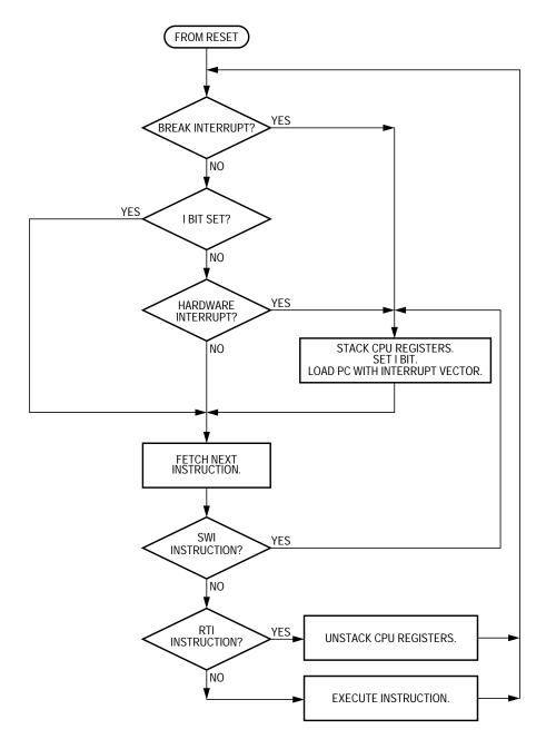
Figure 9-9. Interrupt Processing
