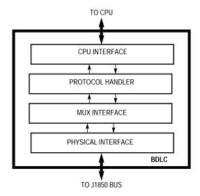
Figure 20-1. BDLC Block Diagram
