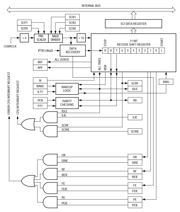
Figure 17-6. SCI Receiver Block Diagram
