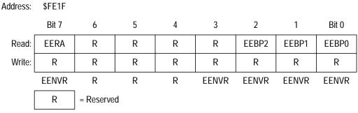
Figure 6-2. EEPROM Array Control Register (EEACR)
