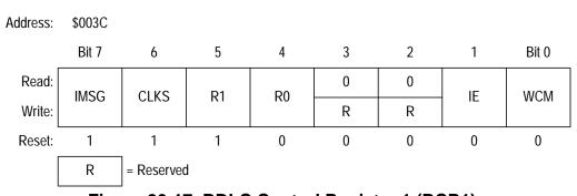
Figure 20-17. BDLC Control Register 1 (BCR1)
