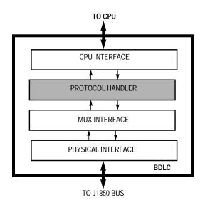
Figure 20-13. BDLC Block Diagram
