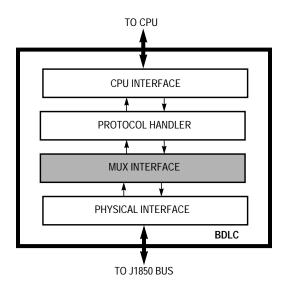
Figure 20-4. BDLC Block Diagram
