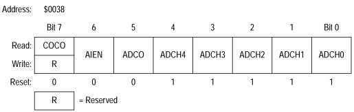
Figure 19-2. ADC Status and Control Register (ADSCR)
