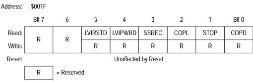
Figure 5-1. Configuration Register (CONFIG)
