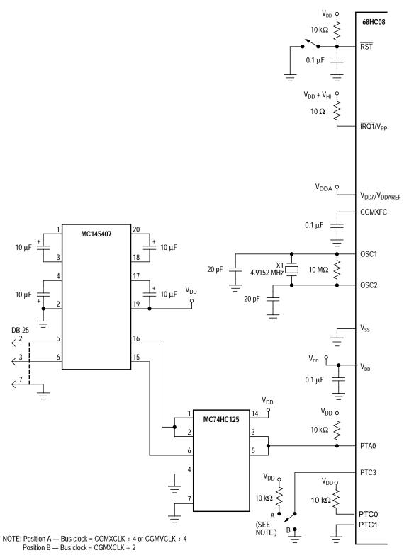
Figure 12-1. Monitor Mode Circuit
