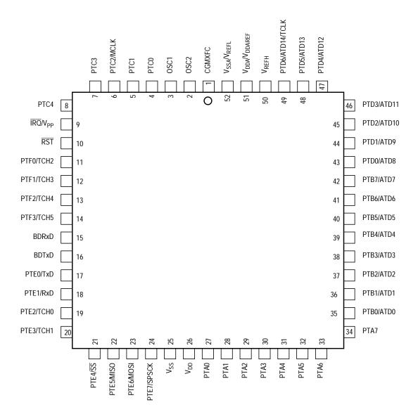
Figure 1-2. 52-Pin PLCC Assignments (Top View)
