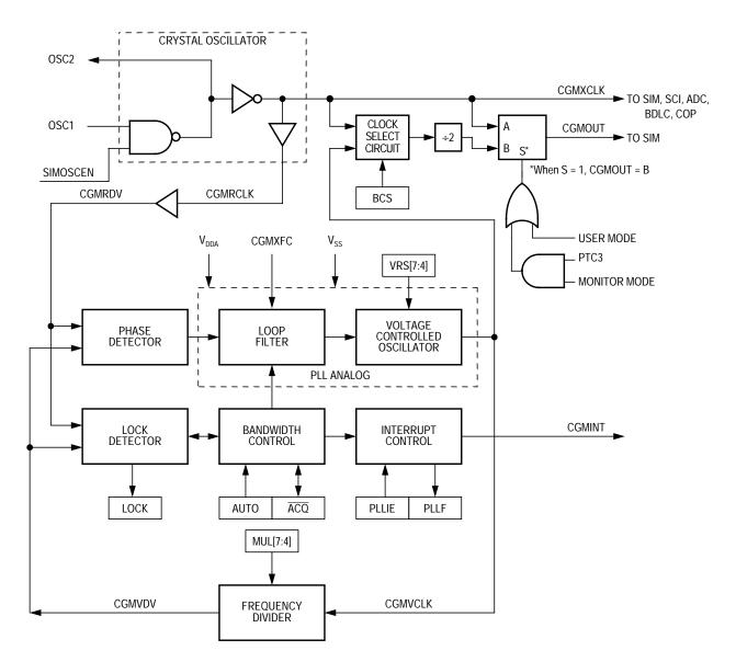
Figure 8-1. CGM Block Diagram
