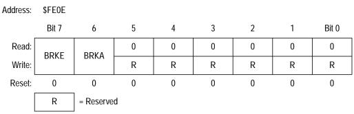
Figure 11-3. Break Status and Control Register (BRKSCR)
