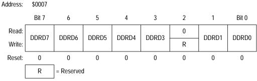
Figure 15-12. Data Direction Register D (DDRD)
