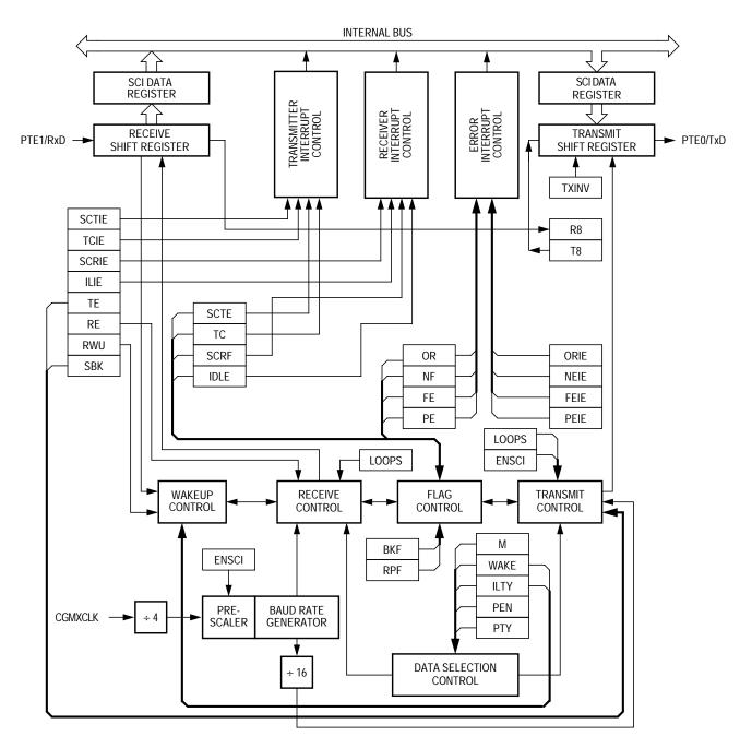
Figure 17-1. SCI Module Block Diagram
