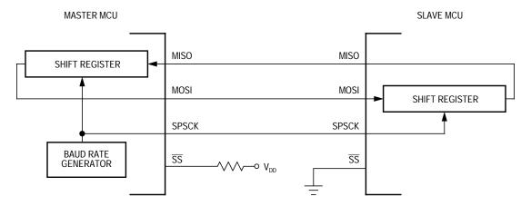
Figure 18-3. Full-Duplex Master-Slave Connections
