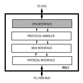
Figure 20-15. BDLC Block Diagram
