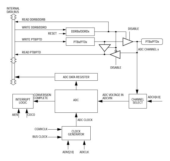
Figure 19-1. ADC Block Diagram
