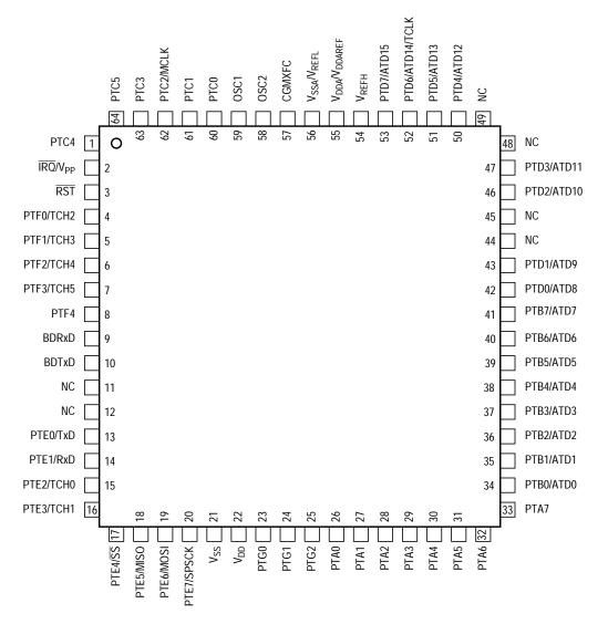
Figure 1-3. 64-Pin QFP Assignments (Top View)
