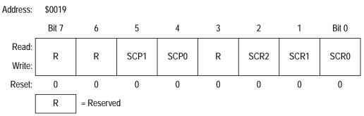
Figure 17-16. SCI BAUD Rate Register 1 (SCBR)
