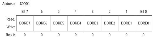
Figure 15-15. Data Direction Register E (DDRE)
