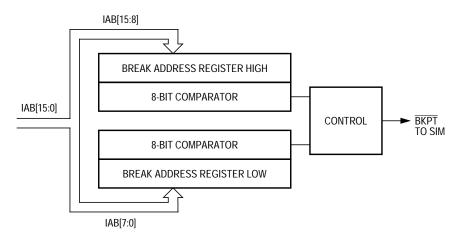
Figure 11-1. Break Module Block Diagram
