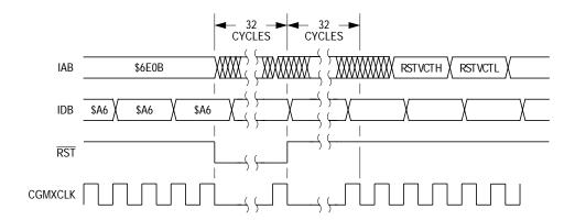
Figure 9-14. Wait Recovery from Internal Reset
