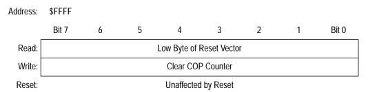
Figure 13-3. COP Control Register (COPCTL)
