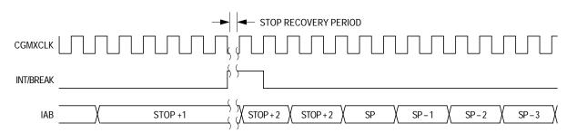
Figure 9-16. Stop Mode Recovery from Interrupt or Break
