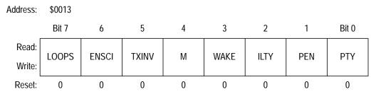
Figure 17-9. SCI Control Register 1 (SCC1)
