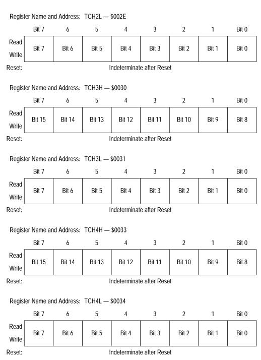
Figure 16-9. TIM Channel Registers (TCH0H/L-TCH3H/L) (Sheet 2 of 3)
