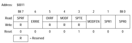
Figure 18-14. SPI Status and Control Register (SPSCR)
