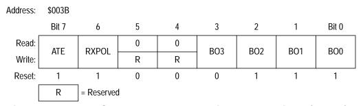
Figure 20-16. BDLC Analog and Roundtrip Delay Register (BARD)
