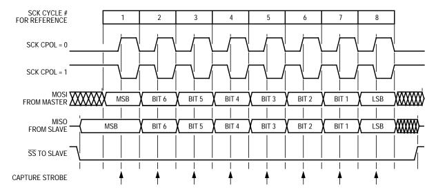
Figure 18-4. Transmission Format (CPHA = 0)
