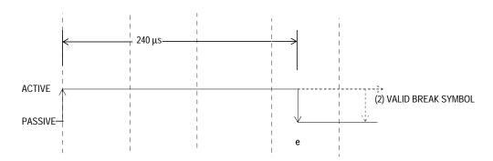
Figure 20-11. J1850 VPW Received BREAK Symbol Times
