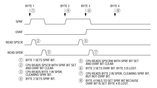
Figure 18-8. Missed Read of Overflow Condition
