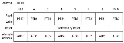
Figure 15-5. Port B Data Register (PTB)
