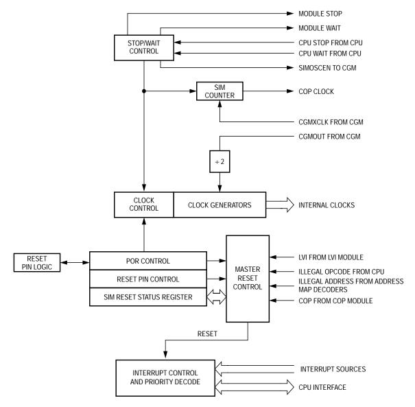
Figure 9-1. SIM Block Diagram
