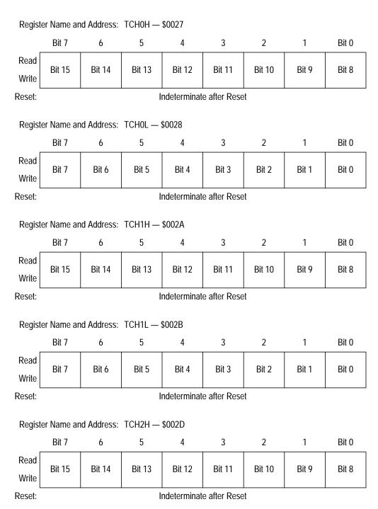
Figure 16-9. TIM Channel Registers (TCH0H/L-TCH3H/L) (Sheet 1 of 3)
