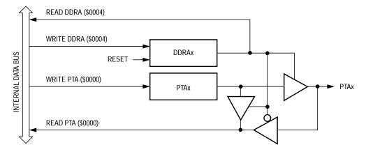
Figure 15-4. Port A I/O Circuit
