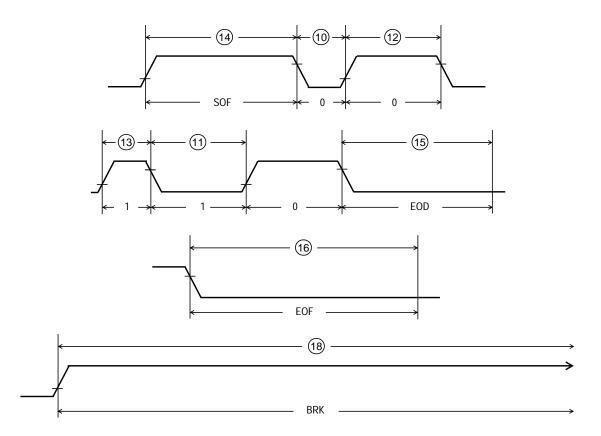
Figure 21-3. BDLC Variable Pulse Width Modulation (VPW) Symbol Timing
