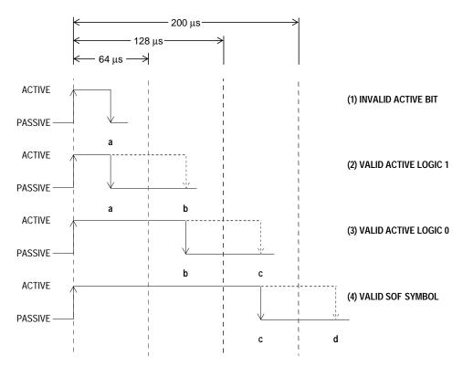
Figure 20-10. J1850 VPW Received Active Symbol Times
