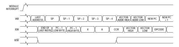
Figure 9-8. Interrupt Entry Timing
