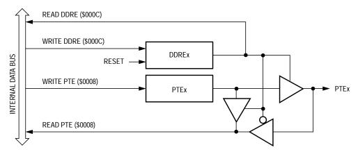
Figure 15-16. Port E I/O Circuit
