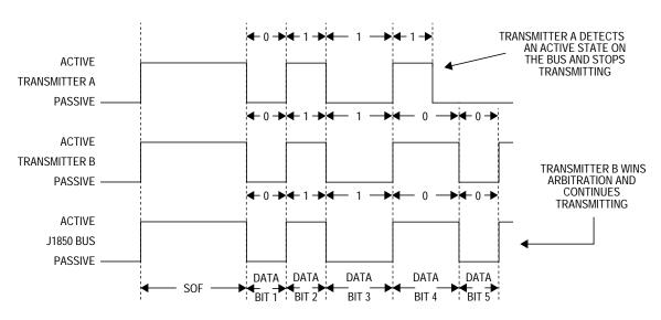
Figure 20-12. J1850 VPW Bitwise Arbitrations
