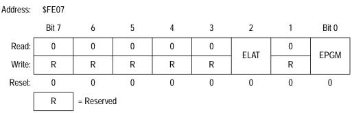
Figure 4-1. EPROM/OTPROM Control Register (EPMCR)
