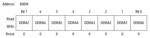
Figure 15-3. Data Direction Register A (DDRA)
