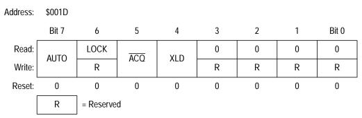
Figure 8-6. PLL Bandwidth Control Register (PBWC)
