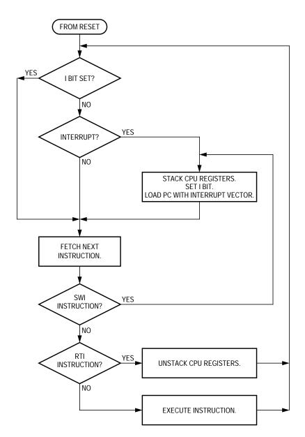
Figure 14-3. IRQ Interrupt Flowchart
