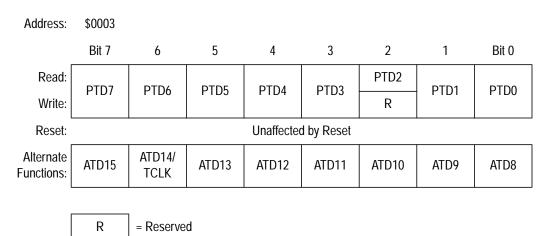
Figure 15-11. Port D Data Register (PTD)
