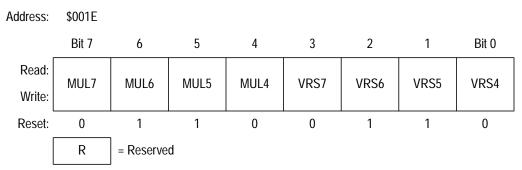
Figure 8-7. PLL Programming Register (PPG)
