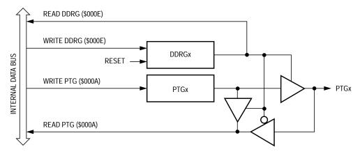
Figure 15-22. Port G I/O Circuit
