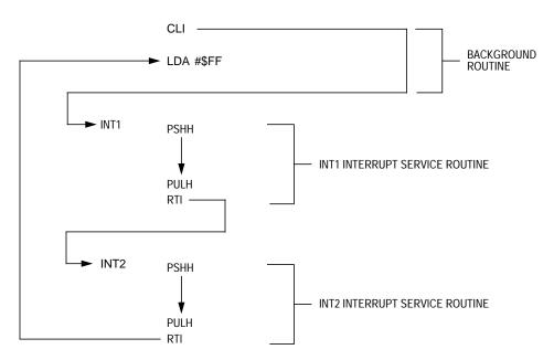
Figure 9-11. Interrupt Recognition Example
