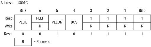
Figure 8-5. PLL Control Register (PCTL)
