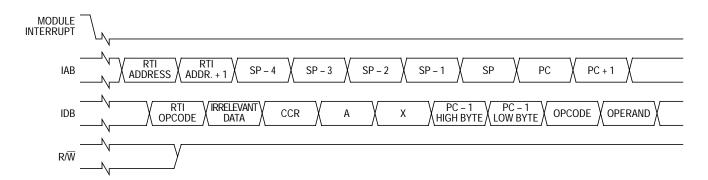
Figure 9-10. Interrupt Recovery Timing
