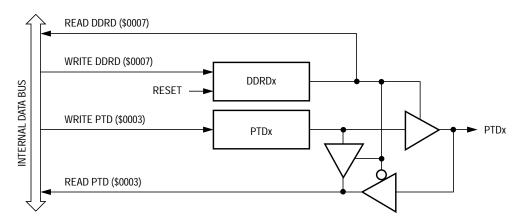
Figure 15-13. Port D I/O Circuit
