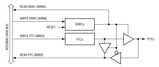
Figure 15-10. Port C I/O Circuit
