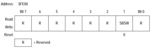
Figure 9-17. SIM Break Status Register (SBSR)
