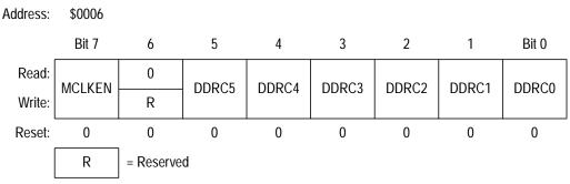
Figure 15-9. Data Direction Register C (DDRC)
