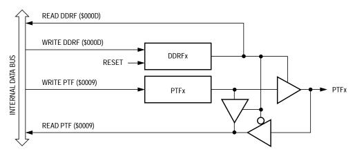
Figure 15-19. Port F I/O Circuit
