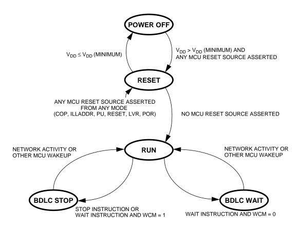
Figure 20-3. BDLC Operating Modes State Diagram
