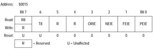
Figure 17-11. SCI Control Register 3 (SCC3)
