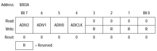
Figure 19-4. ADC Input Clock Register (ADICLK)
