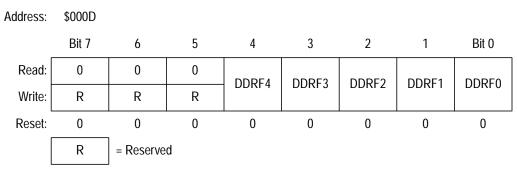
Figure 15-18. Data Direction Register F (DDRF)
