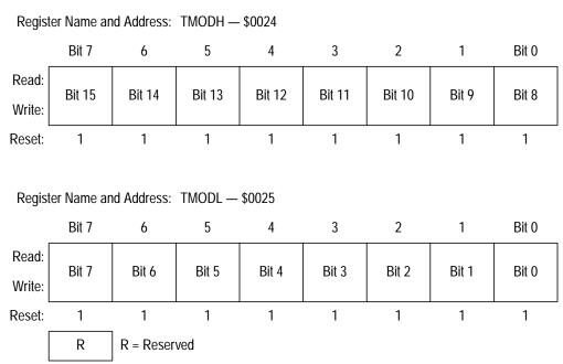
Figure 16-6. TIM Counter Modulo Registers (TMODH and TMODL)
