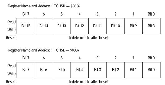
Figure 16-9. TIM Channel Registers (TCH0H/L-TCH3H/L) (Sheet 3 of 3)
