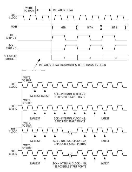
Figure 18-7. Transmission Start Delay (Master)
