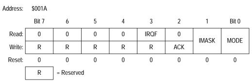
Figure 14-4. IRQ Status and Control Register (ISCR)
