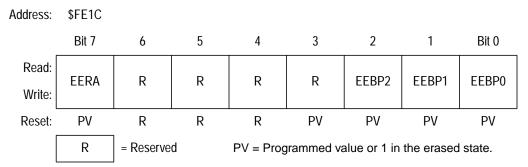
Figure 6-3. EEPROM Non-Volatile Register (EENVR)
