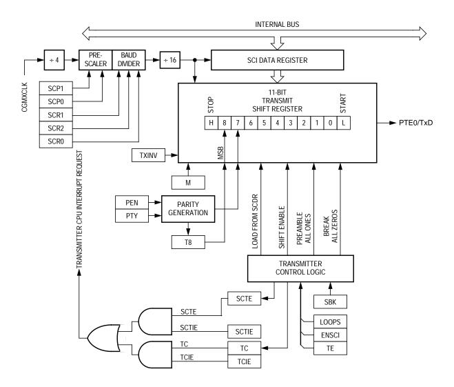
Figure 17-4. SCI Transmitter
