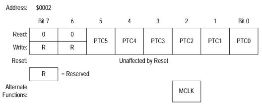
Figure 15-8. Port C Data Register (PTC)
