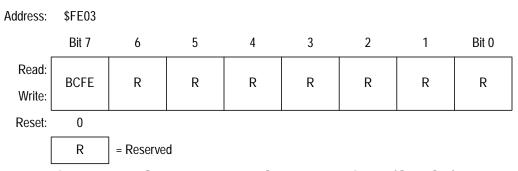
Figure 9-19. SIM Break Flag Control Register (SBFCR)
