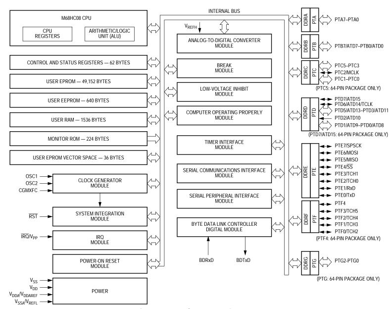
Figure 1-1. MCU Block Diagram
