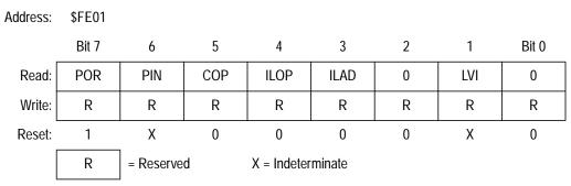
Figure 9-18. SIM Reset Status Register (SRSR)
