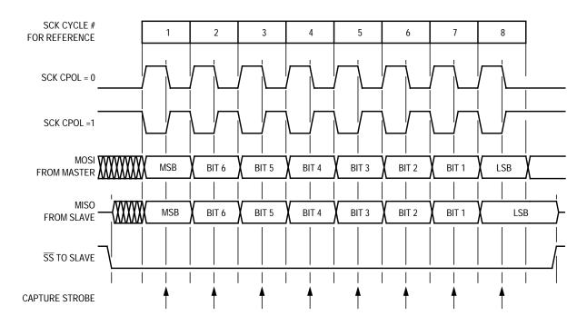
Figure 18-6. Transmission Format (CPHA = 1)
