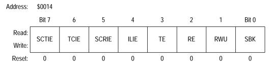
Figure 17-10. SCI Control Register 2 (SCC2)
