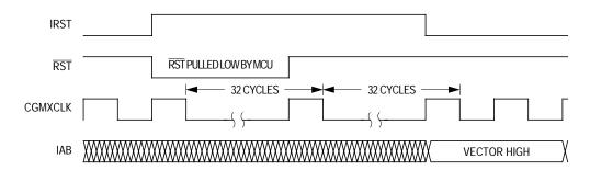
Figure 9-5. Internal Reset Timing
