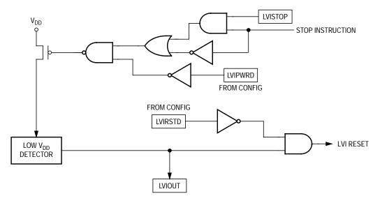
Figure 10-1. LVI Module Block Diagram
