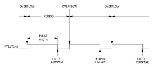
Figure 16-3. PWM Period and Pulse Width
