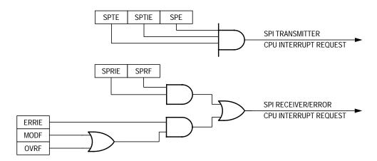
Figure 18-10. SPI Interrupt Request Generation
