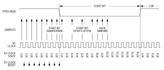
Figure 17-8. Receiver Data Sampling
