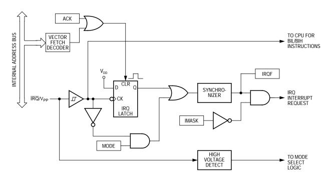
Figure 14-1. IRQ Block Diagram
