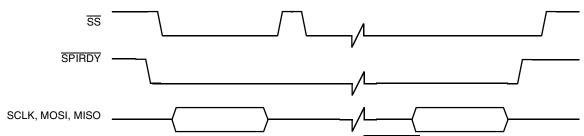
Figure 7. Master CSPI Timing Diagram Using SPI\_RDY Level Trigger
