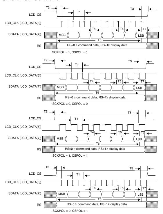
Figure 15. SLCDC Serial Transfer Timing
