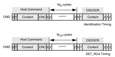
Figure 18. Timing Diagrams at Identification Mode
