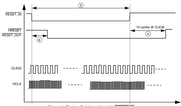
Figure 3. Timing Relationship with RESET\_IN
