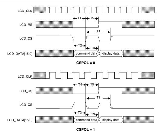
Figure 16. SLCDC Parallel Transfers Timing
