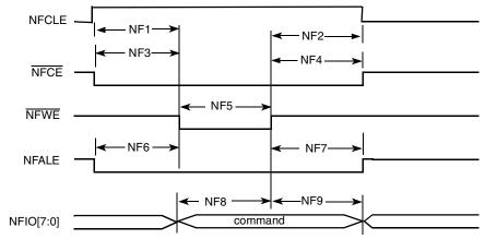
Figure 25. Command Latch Cycle Timing Dlagram
