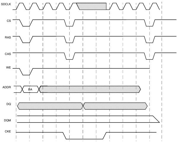
Figure 33. SDRAM Self-Refresh Cycle Timing Diagram
