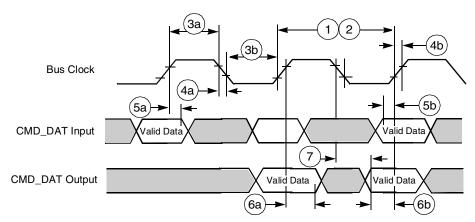
Figure 17. Chip-Select Read Cycle Timing Diagram
