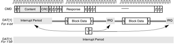
Figure 23. SDIO IRQ Timing Diagram
