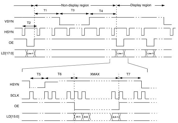
Figure 12. 4/8/12/16/18 Bit/Pixel TFT Color Mode Panel Timing
