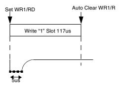
Figure 40. Write 1 Timing
