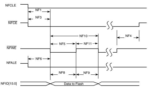
Figure 27. Write Data Latch Timing Dlagram
