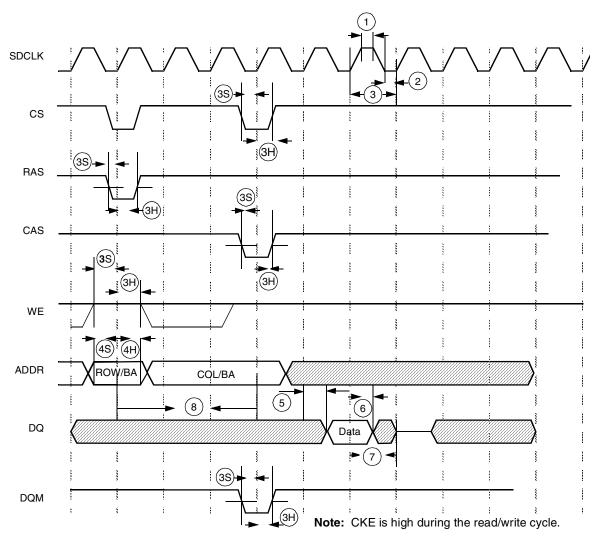
Figure 30. SDRAM Read Cycle Timing Diagram
