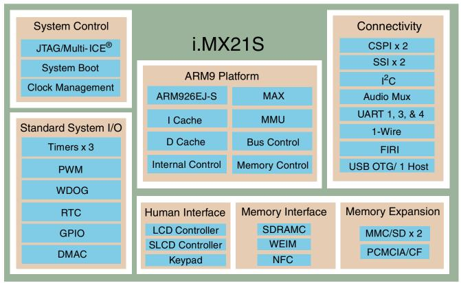
Figure 1. i.MX21S Functional Block Diagram
