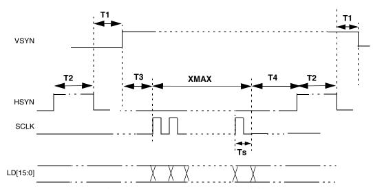
Figure 14. Non-TFT Mode Panel Timing
