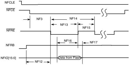
Figure 28. Read Data Latch Timing Diagram
