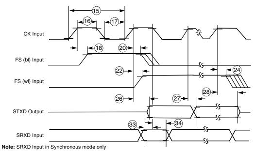
Figure 36. SSI Transmitter External Clock Timing Diagram
