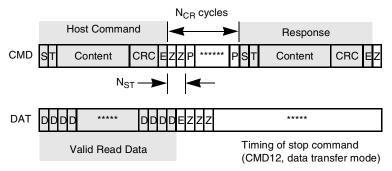
Figure 20. Timing Diagrams at Data Read
