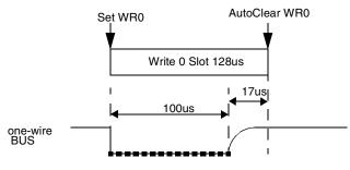
Figure 39. Write 0 Timing
