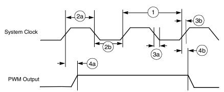
Figure 29. PWM Output Timing Diagram
