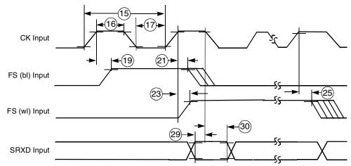
Figure 37. SSI Receiver External Clock Timing Diagram
