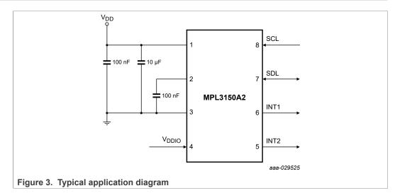
The device power is supplied through the V<sub>DD</sub> line. Power supply decoupling capacitors (100 nF ceramic plus 10 µF bulk or 10 µF ceramic) should be placed as near as possible to pin 1 of the device. A second 100 nF capacitor is used to bypass the internal regulator. The functions, threshold, and the timing of the interrupt pins (INT1 and INT2) are user programmable through the I<sup>2</sup>C interface.
