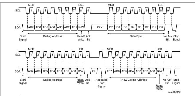
Figure 5. I<sup>2</sup>C bus transmission signals
