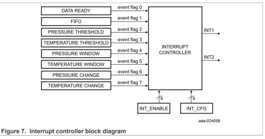
The system's interrupt controller uses the corresponding bit field in the CTRL\_REG5 register to determine the routing table for the INT1 and INT2 interrupt pins. If the bit value is logic '0' the functional block's interrupt is routed to INT2, and if the bit value is logic '1' then the interrupt is routed to INT1.
