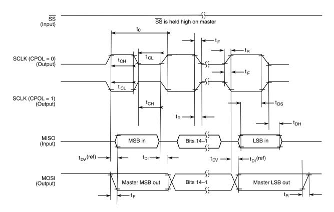
Figure 18. SPI Master Timing (CPHA = 1)
