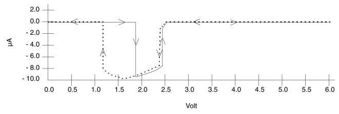
Figure 11. I<sub>IN</sub>/I<sub>OZ</sub> versus V<sub>IN</sub> (Typical; Pull-Up Disabled)
