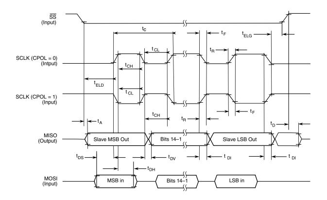
Figure 19. SPI Slave Timing (CPHA = 0)
