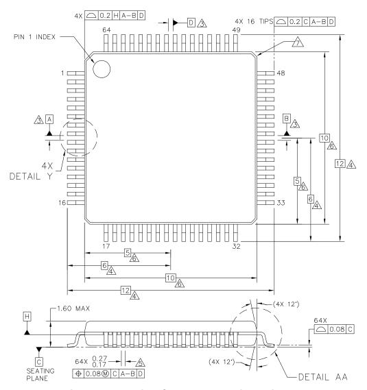
Figure 29. 64-pin LQFP package dimensions 1
