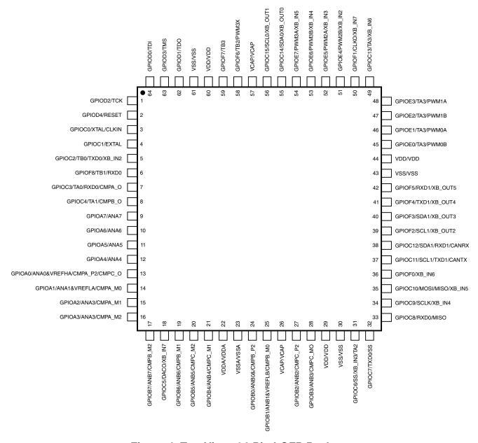
Figure 4. Top View: 64-Pin LQFP Package
