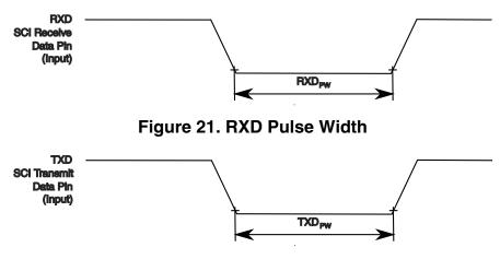
Figure 22. TXD Pulse Width
