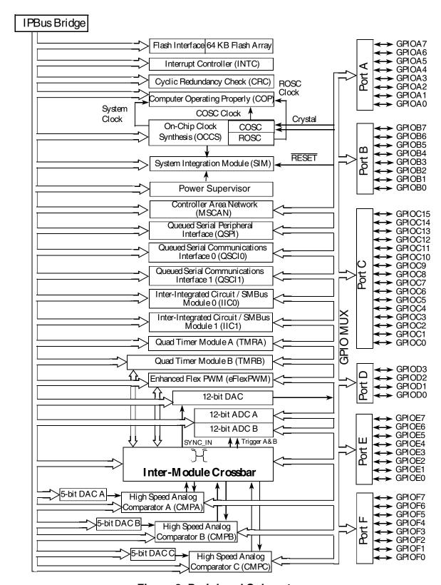
Figure 3. Peripheral Subsystem
