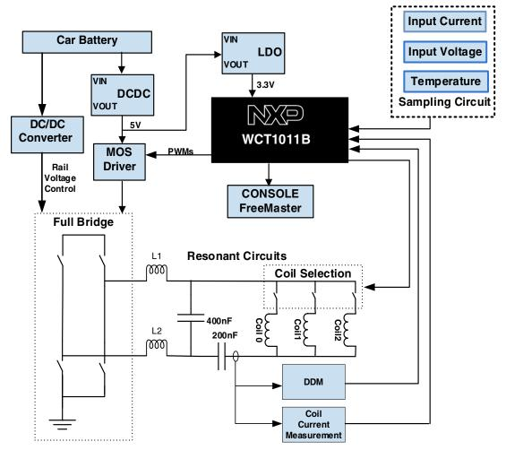
Figure 1. Wireless Charging System Functional Diagram
