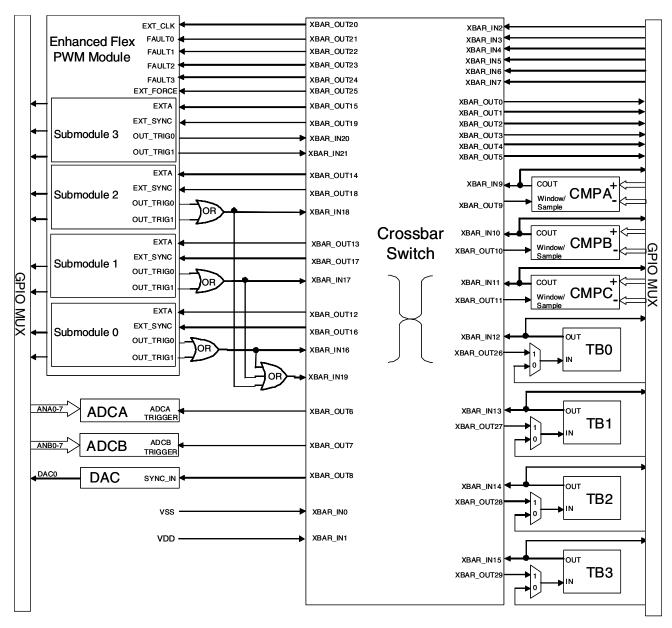
Figure 10. Crossbar Switch Connections
