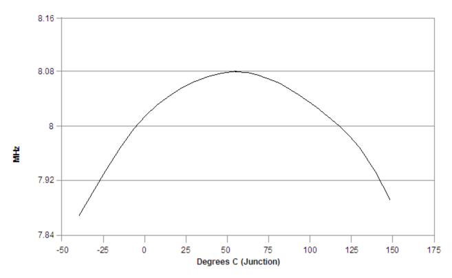
Figure 15. Relaxation Oscillator Temperature Variation (Typical) After Trim
