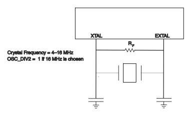
Figure 7. Typical Crystal or Ceramic Resonator Circuit
