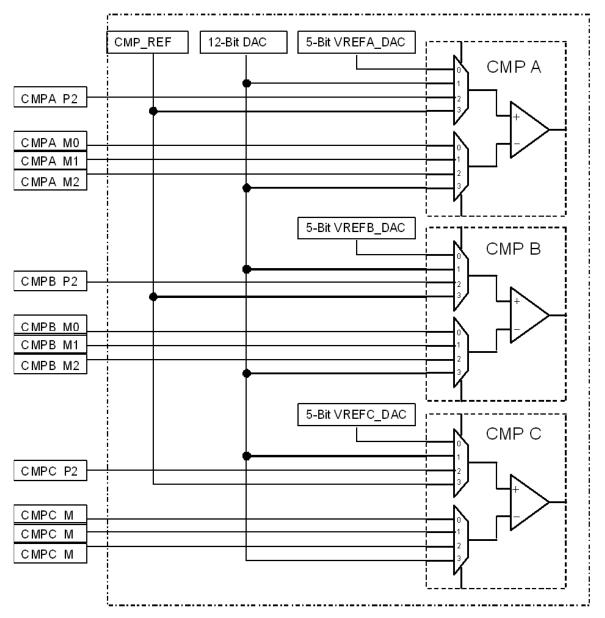
Figure 9. On-Chip Comparator Connections
