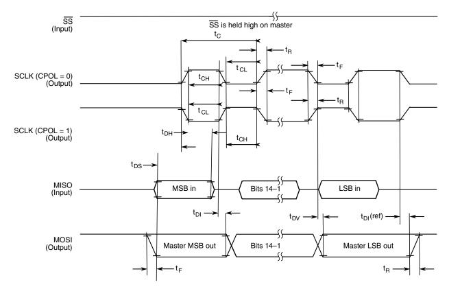
Figure 17. SPI Master Timing (CPHA = 0)
