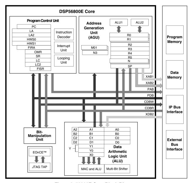
Figure 2. 56800E Core Block Diagram
