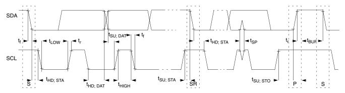
Figure 24. Timing Definition for Fast and Standard Mode Devices on the I<sup>2</sup>C Bus
