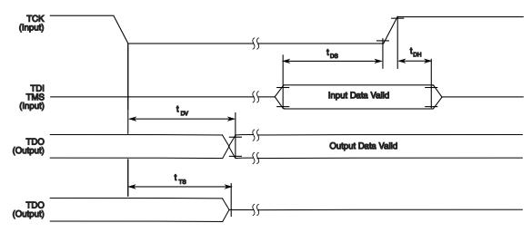
Figure 26. Test Access Port Timing Diagram
