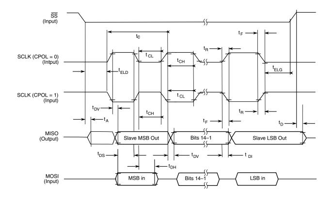
Figure 20. SPI Slave Timing (CPHA = 1)
