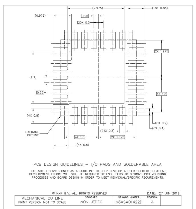
Figure 28. Reflow soldering footprint part2 for HQFN24 (SOT1931-1(D))
