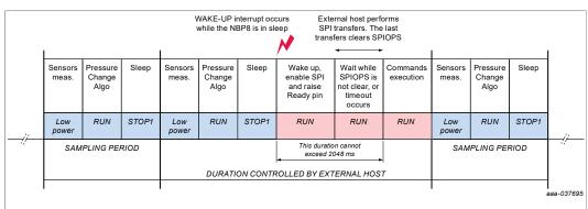
Figure 23. External host requests SPI transfers and then clears the SPIOPS register
