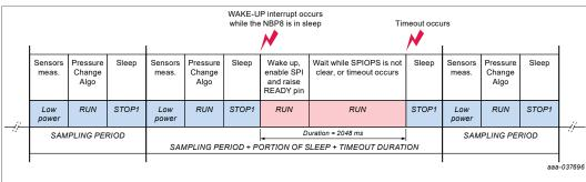
Figure 24. External host requests SPI transfers but does not clear the SPIOPS register
