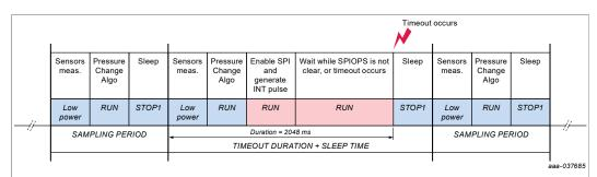
Figure 22. Sequence of events when NBP8 notifies the external host of an event but the external host does not clear the SPIOPS register
