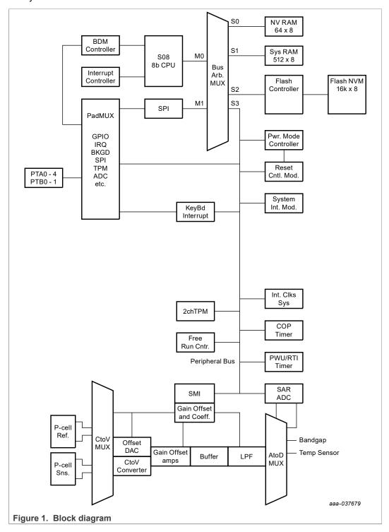
**Battery pressure monitor sensor**
