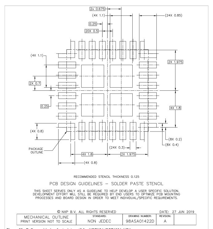
Figure 29. Reflow soldering footprint part3 for HQFN24 (SOT1931-1(D))
