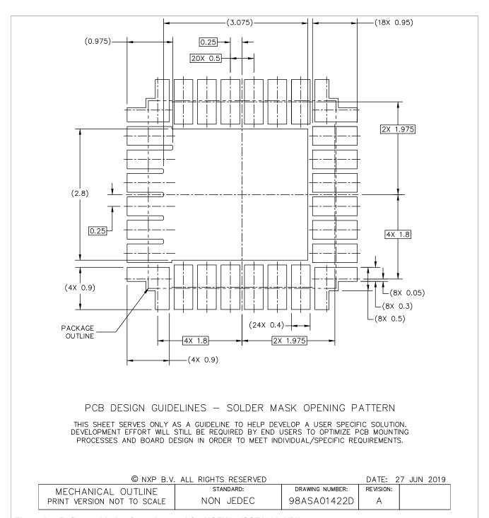
Figure 27. Reflow soldering footprint part1 for HQFN24 (SOT1931-1(D))
