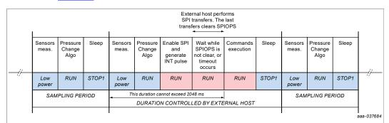
Figure 21. Sequence of events when NBP8 notifies the external host of an event and the external host clears the SPIOPS register
