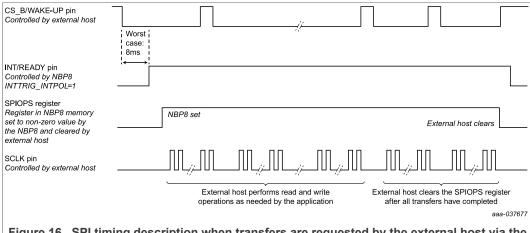
Figure 16. SPI timing description when transfers are requested by the external host via the WAKE-UP pin, with INTTRIG\_INTPOL=1
