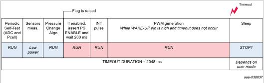
Figure 28. Sequence of events when an event requiring attention occurs and the external host does not request SPI transfers within the timeout limit
