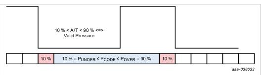
Figure 20. Duty cycle between 10 % and 90 %, with CFGMODE\_PWMPOL=0
