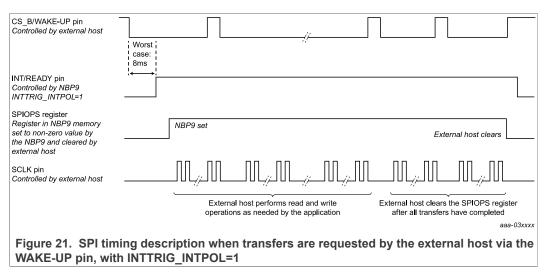
**Note:** <u>Figure 21</u> shows that the CS\_B / WAKE-UP pin is held low by the external host from the moment the external host lowers the pin to request a transfer, until the end of the first SPI transfer. In reality, the actual sequence implemented by the external host may be different, taking into account the possible software implementation described below.
