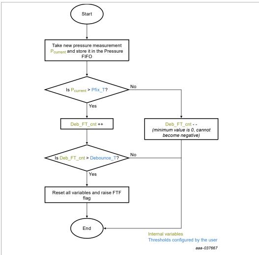
Figure 9. Fixed Threshold algorithm flow
