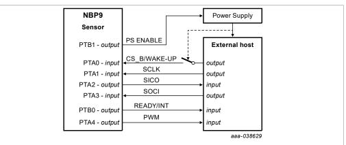
Figure 4. Connections between the NBP9 and external host
