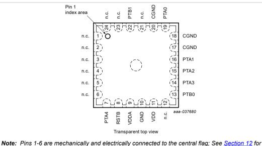
**Note:** Pins 1-6 are mechanically and electrically connected to the central flag; See <u>Section 12</u> for details. If additional ground is desired, any of the pins 1-6 may be routed to circuit board ground plane, or the central flag may be connected to circuit board ground plane with vias.
