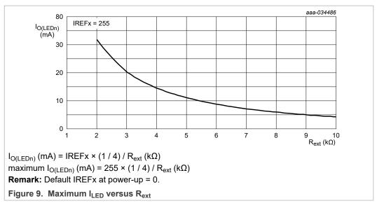
**Example 1:** If  $R_{ext} = 2 k\Omega$ ,  $I_0\_LED\_MIN = 125.0 \mu A$ ,  $I_0\_LED\_MAX = 31.875 mA$  (as shown in Figure 10).
