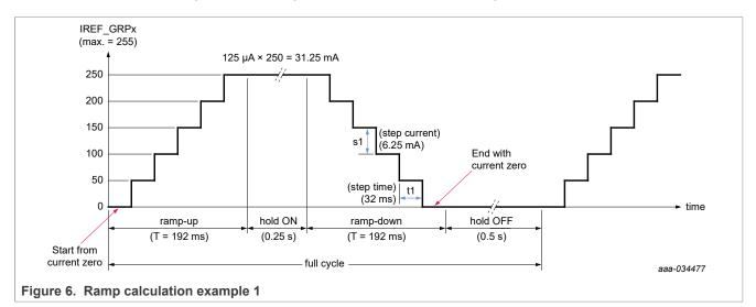
7.2.8.8 Ramp control — equation and calculation example
