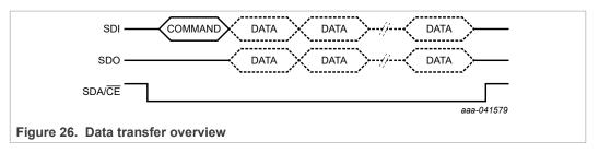
The command byte defines the address of the first register to be accessed and the read/ write mode. The address counter will auto increment after every access and will reset to zero after the last valid register is accessed. The R/W bit defines if the following bytes are read or write information.
