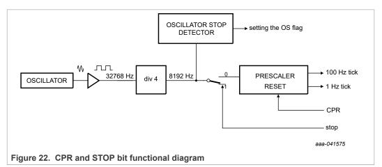
The *stop* signal blocks the 8.192 kHz clock from generating system clocks and freezes the time. In this state, the prescaler can be cleared with the CPR command in the Resets register.
