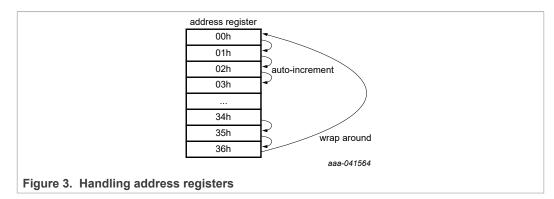
• The first five registers (memory address 00h, 01h, 02h, 03h and 04h) are used as control registers (see <u>Section 7.2</u>).
