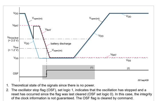
Figure 8. Power failure event due to battery discharge: reset occurs
