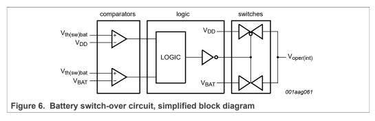
$V_{oper(int)}$  is at  $V_{DD}$  or  $V_{BAT}$  potential.
