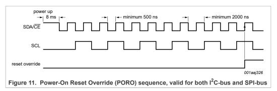
Once the override mode is entered, the device is immediately released from the reset state and the set-up operation can commence.
