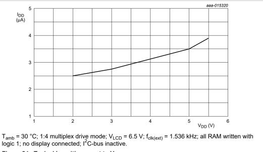
Figure 24. Typical  $I_{\text{DD}}$  with respect to  $V_{\text{DD}}$
