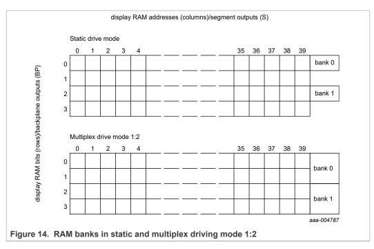
There are two banks; bank 0 and bank 1. Figure 14 shows the location of these banks relative to the RAM map. Input and output banks can be set independently from one another with the Bank-select command (see Table 9). Figure 15 shows the concept.
