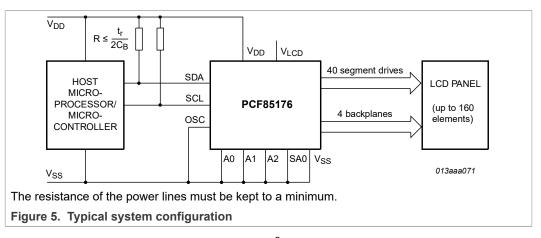
The host microcontroller maintains the 2-line  $I^2$ C-bus communication channel with the PCF85176. The internal oscillator is enabled by connecting pin OSC to pin V<sub>SS</sub>. The appropriate biasing voltages for the multiplexed LCD waveforms are generated internally.
