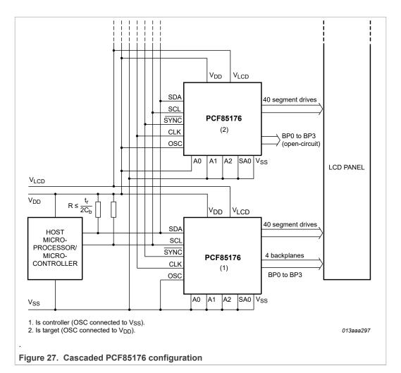
The <u>SYNC</u> line is provided to maintain the correct synchronization between all cascaded PCF85176. Synchronization is guaranteed after a power-on reset. The only time that <u>SYNC</u> is likely to be needed is if synchronization is accidentally lost (e.g. by noise in adverse electrical environments or by defining a multiplex drive mode when PCF85176 with different SA0 levels are cascaded).
