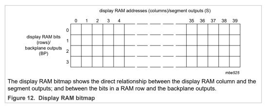
When display data is transmitted to the PCF85176, the display bytes received are stored in the display RAM in accordance with the selected LCD drive mode. The data is stored as it arrives and depending on the current multiplex drive mode the bits are stored singularly, in pairs, triples, or quadruples. To illustrate the filling order, an example of a 7-segment display showing all drive modes is given in Figure 13. The RAM filling organization depicted applies equally to other LCD types.
