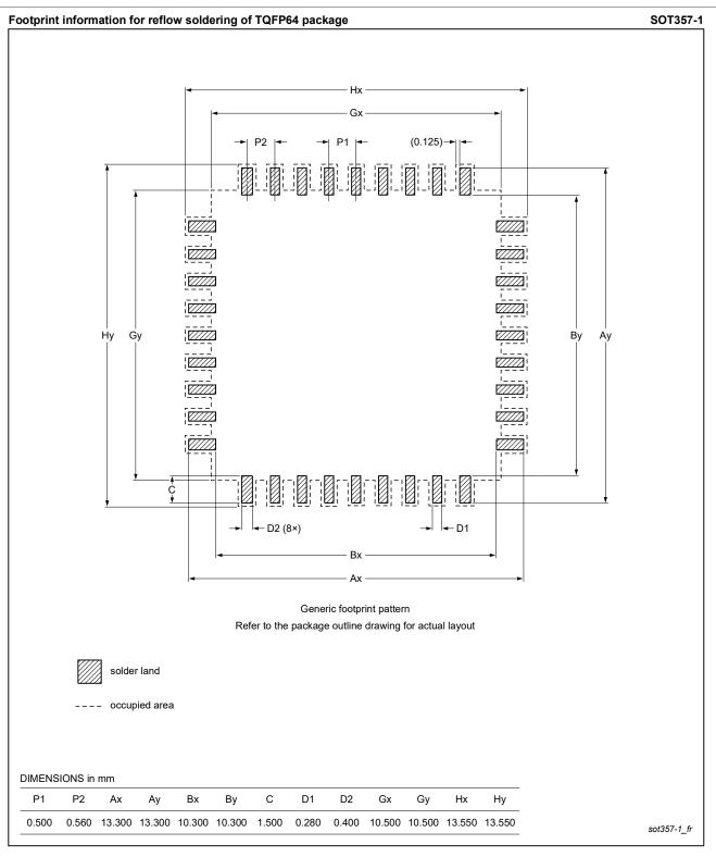
Figure 32. Footprint information for reflow soldering of SOT357-1 (TQFP64) of PCF85176H
