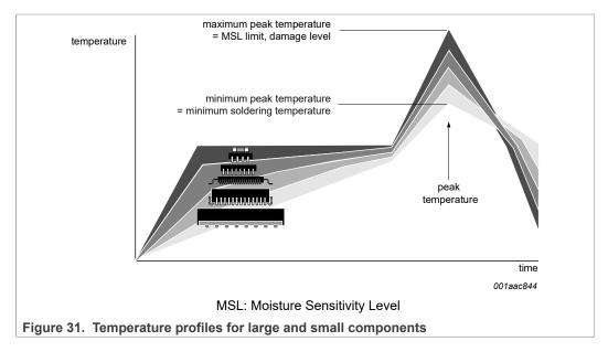
Studies have shown that small packages reach higher temperatures during reflow soldering, see <u>Figure 31</u>.
