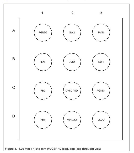
Dual Synchronous 1.5A/1.5A Step-down Buck Regulators with 525 mA LDO
