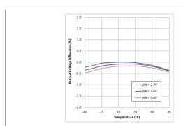
Figure 41. Buck1 Output Voltage Error vs Temperature
