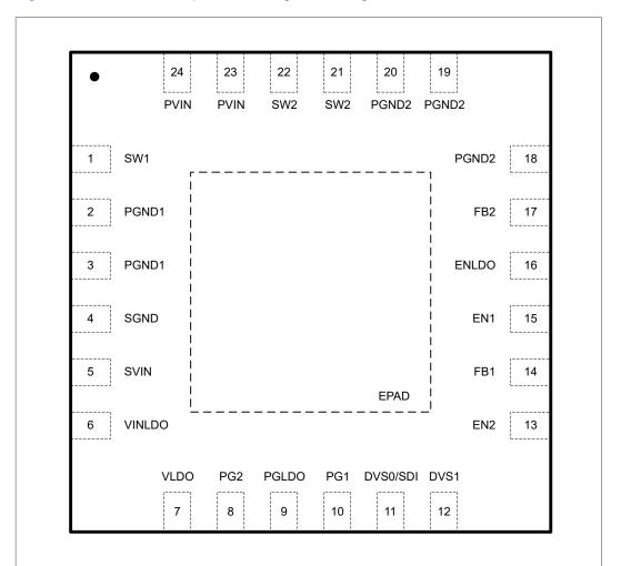
Figure 5. 4 mm x 4 mm QFN-24 in 0.5 mm pitch pin configuration, top (see through) view
