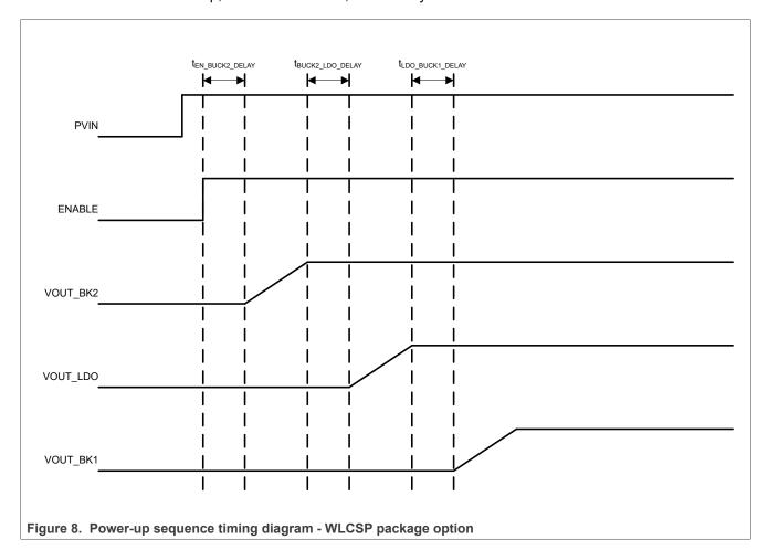
Dual Synchronous 1.5A/1.5A Step-down Buck Regulators with 525 mA LDO
