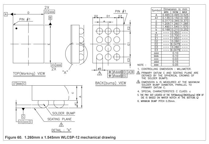
**Note:** All dimensions in mm. See <u>Section 9.2 "Package markings"</u> for package marking and pin 1 location.
