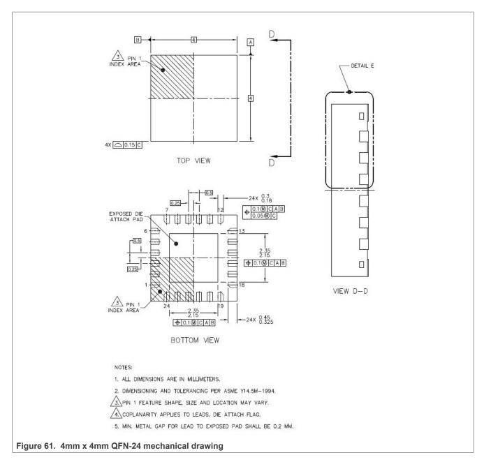
**Note:** All dimensions in mm. See <u>Section 9.2 "Package markings"</u> for package marking and pin 1 location.
