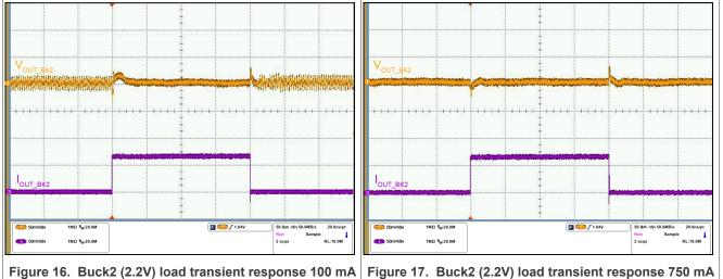
Figure 16. Buck2 (2.2V) load transient response 100 mA to 750 mA
