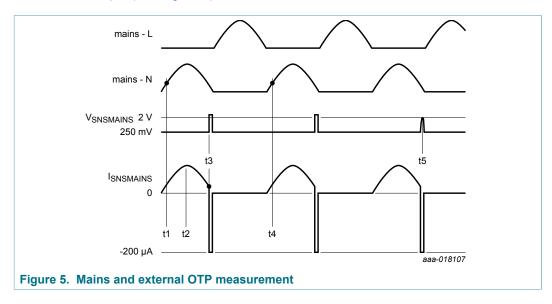
At t1, the voltage at the SNSMAINS pin is internally regulated to  $V_{regd(SNSMAINS)}$  (250 mV). The current into the SNSMAINS pin is a measure of the system input mains voltage. The TEA19162HT continuously measures the SNSMAINS current and waits until it detects a peak in the measured current (t2). This peak current value is internally stored and used as an input for the brownout/brownin detection and the mains compensation.
