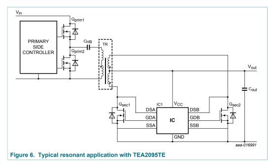
GreenChip dual synchronous rectifier controller
