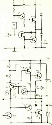
Fig. 2. Circuit chosen to allow feedback control of the operating current.
