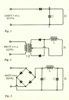
small in each case, the maximum reverse voltage appearing across each diode is:
