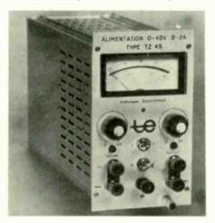
and fine adjustment controls. Unit measures  $4 \times 7 \times 11\frac{1}{2}$ in. An over-voltage crowbar with operating time of less than 20µs, operating temperature range of 0-60°C, ripple 300µV r.m.s. and load and line regulation 1 part in 10,000 is available as an optional extra. Tranchant Electronics (U.K.) Ltd, 17 Charing Cross Road, London. W.C.2.
