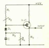
Modified unijunction transistor oscillator.
