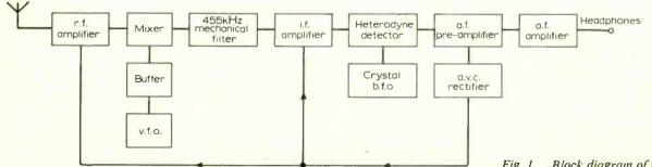
Fig. 1. Block diagram of the complete receiver.
