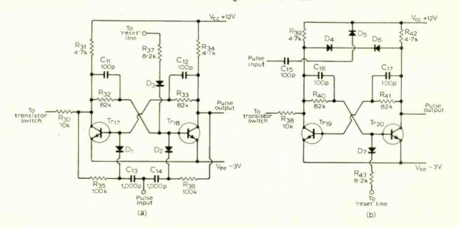
Fig. 4 (a). First bistable. Diodes are germanium types, e.g. OA81, OA91, IN914.  $Tr_{17}$  and  $Tr_{18}$  can be 2N3708, BC108, etc. (b). Circuit for remaining five bistables. Diodes and transistors as for first bistable.
