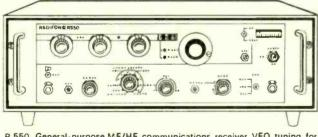
R.550. General-purpose MF/HF communications receiver. VFO tuning for search with a resolution of 10 Hz, and frequency synthesis with 100 Hz increments for accurate setting to known frequencies. Dynamic range exceeds 120 dB, with superb blocking and cross modulation characteristics. Stringent defence specification at realistic price for commercial users.
