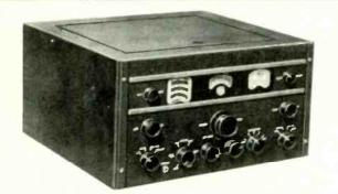
BRAND NEW and in original cases-A.C. mains input. 110V 2.5-600 ohms. Complete with crystal filter, noise limiter, B.F.O., H.F. tone control, R.F. & A.F. variable controls. Price £87/10/each, carr. £2.
