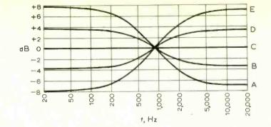
Fig. 2. Calculated frequency response of tone balance control circuit shown in Fig. 1(a).  $A-R_2 = 0, R_3 = 100 \text{ k}\Omega; B-R_2 = 25 \text{ k}\Omega; R_3 = 75 \text{ k}\Omega; C-R_2 = R_3 = 50 \text{ k}\Omega;$  $D-R_2 = 75 \text{ k}\Omega, R_3 = 25 \text{ k}\Omega; \text{ and } E-R_2 = 100 \text{ k}\Omega, R_3 = 0.$
