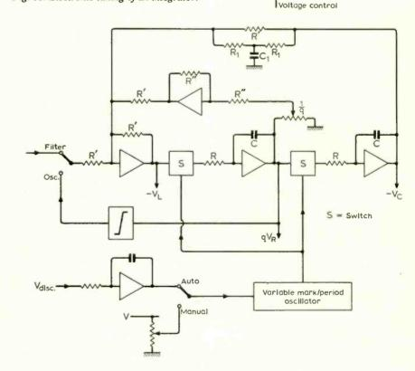
Fig. 12. Electronic tuning applied to a two-integrator system.
