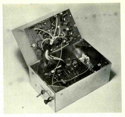
The components of the digitally-controlled pre-amp. need take up little space—the aluminium case shown measures only  $6in \times 4in \times 2\frac{1}{2}in$ . The bistables are mounted on the board attached to the lid of the container, the other board carrying the amplifier and the peak-level sensor. Amplifier input and output are carried by screened leads. The bunch of unscreened leads joining pulse counter to the amplifier carries switching signals only. The power supply is external.
