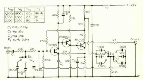
Low-pass and high-pass filter circuit.
