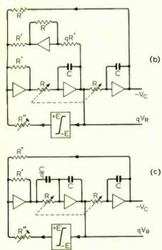
Fig. 8. Two-phase low-frequency oscillator.
