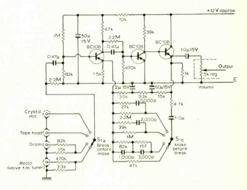
Fig. 3. Input stage (modified Bailey).
