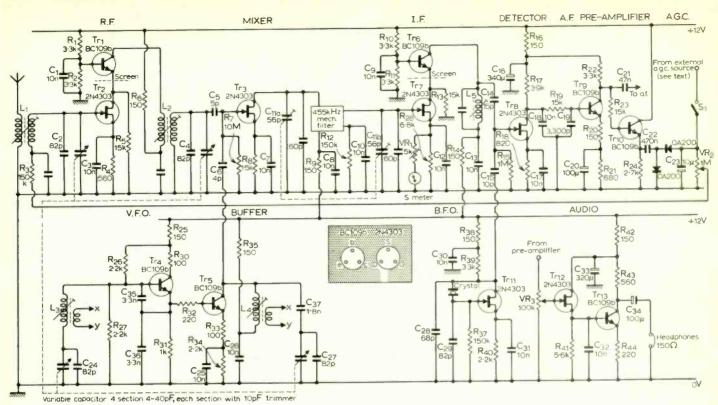
Fig. 2. The circuit. A power supply is not included in this description, but a car battery or almost any mains 12V power pack will suffice.
