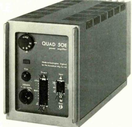
**INPUTS** – 0.5 Vrms unbalanced with provision for an optional plug-in transformer for bridging 600 ohms lines. **OUTPUTS** – isolated providing 50 watts into almost any impedance from 4 to 200 ohms. **DIMENSIONS** –  $12\frac{3}{4}^{"} \times 6\frac{1}{4}^{"} \times 4\frac{1}{2}^{"}$
