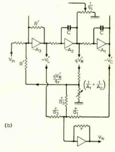
Fig. 1. (a) Ideal two-integrator system. (b) Showing a method of correcting Q factor and notch response when integrators have finite gain.
