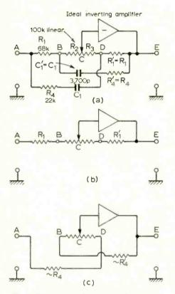
Fig. 1. Basic tone balance control system (a); exact equivalent at low frequencies (b); and approximate equivalent at high frequencies (c).
