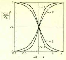
Fig. 6. Power responses of 2nd- and 3rdorder crossover filters with Butterworth response.
