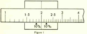
The spacing of the tolerance marks on the cursor is correct for any point on the scale and can be extended to include a range of tolerances in addition to the 10% marks illustrated.
