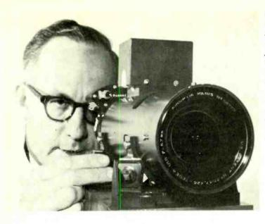
One of the TV cameras used in the satellite TIROS-M which is now providing weather information for the world's meteorological centres. TIROS-M was built by R.C.A. under the direction of N.A.S.A's Goddard Space Flight Centre
