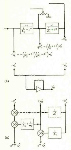
Fig. 3. (a) Analysis of system with finite-gain integrators. (b) Method of compensation.
