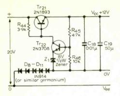
Fig. 5. A suitable power supply.
