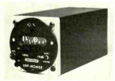
operation, the emergency channel is preset to the v.h.f. or u.h.f. international aviation distress frequency; an auxiliary channel can be used to within  $\pm 2.5$ MHz (v.h.f.) or  $\pm 5$ MHz (u.h.f.) for training and/or tactical purposes. The homer provides 'left/right' indications from the received signal. Audio outputs to the aircraft intercom system are provided. The unit costs under  $\pm 500$ , plus installation. Burndept Electronics (E.R.) Ltd, St. Fidelis Road, Erith, Kent.
