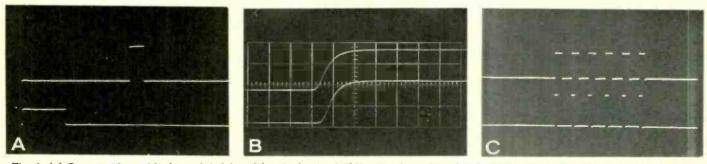
Fig. 1. (a) Output pulses with channel A delayed (vertical gain: 2V/div.; timebase:  $10\mu s/div.$ ). (b) Rise time of both channels showing that time coincidence can be achieved (Vertical gain: 2V/div.; time base: 50ns/div.). (c) The action of the inhibit pulse (vertical gain: 2V/div.; timebase: 0.5ms/div.).
