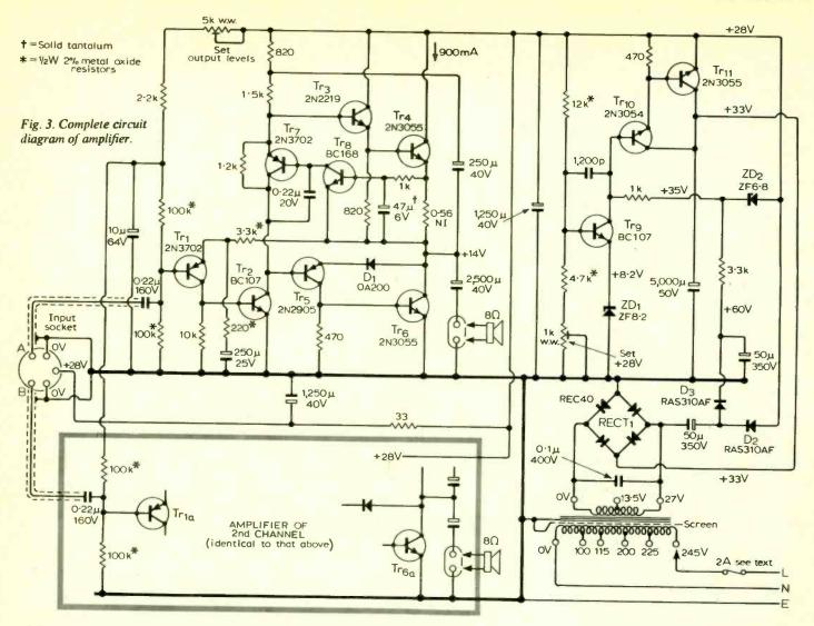
The main supply is a normal bridge rectifier with capacitance smoothing. The value of this capacitor is decided by the maximum permissible ripple, which in turn depends on the minimum mains voltage allowable and the minimum voltage across the regulator series transistors at which the regulator still retains full control.
