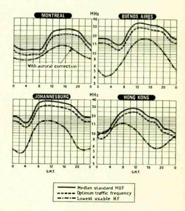
The charts show median standard MUF, optimum traffic frequency (FOT) and lowest usable frequency (LUF) for reception in this country. LUFs were calculated by Cable & Wireless Ltd for specific point-to-point telegraph circuits. LUFs for domestic reception of high-power broadcast transmissions would be slightly higher and those for the amateur bands considerably higher, especially during daylight.
