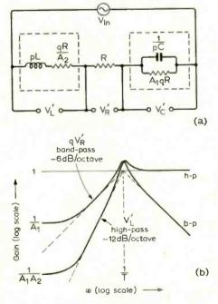
Fig. 4. (a) Equivalent circuit of system with finite-gain integrators. (b) Uncompensated responses.
