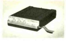
moving parts. The output power is 5–7 watts, and receiver sensitivity is  $0.5_{\mu}$ V to open squelch. Audio output is 2.5 watts into 3Q. Power requirements (from 12V vehicle battery) is 1.9A on transmit (full modulation) and 0.2A on standby. Standard Telephones and Cables Ltd, S.T.C. House, 190 Strand, London, W.C.2.
