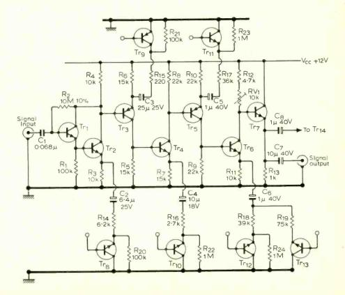
considerably improved. The maximum distortion occurred at unity voltage gain and was less than 0.05% for an output of 1V r.m.s. For a heavy overload the gain reduced at the rate of 4000dB per second and the greatest gain reduction step was less than 2dB. The prototype was constructed for less than £5 10s using components as advertised in *Wireless World* and was placed in an aluminium box measuring approx.  $100 \times 150 \times 65 \text{ mm} (4 \times 6 \times 2\frac{1}{2} \text{ in}).$
