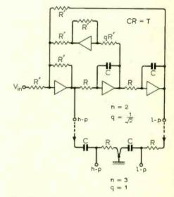
Fig. 7. Two-integrator system as crossover filter.
