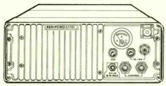
GA.481. 100-watt linear amplifier, broad-band 1.5-30 MHz. No tuning or loading. Automatic protection against any mismatch (from open- to shortcircult aerial) or excessive drive. Easily portable, will operate direct from vehicle supply.
