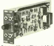
Output capability is  $\pm 8V$  at up to 1.5mA and common mode rejection is greater than 100dB. Full shift of the output is possible, and wideband noise is less than 10mV pk-pk, referred to output. Bandwidth may be adjusted, from d.c. to between 100Hz and 100kHz. A monolithic input stage produces drift performance better than  $5_u V/^{\circ}C$ , referred to input. Fylde Electronic Laboratories Ltd, 6/16 Oakham Court, Preston, PR 1 3XP.
