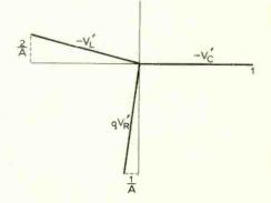
Fig. 2. Relative phases of three primary responses at  $\omega_c$ .
