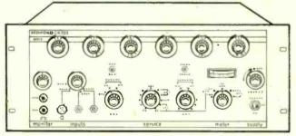
GK.203. Frequency synthesis drive unit. 1.5-30 MHz in 100 Hz increments 17 modes of transmission, including ISB if specified.
